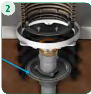
2 Remove Lower Bolts and Ring and Remove Bellows
