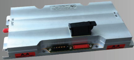
Module -0 Conduction through baseplate
