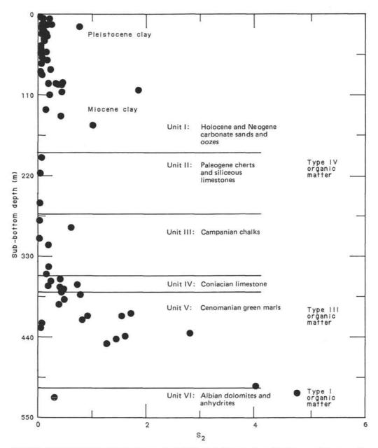
Figure 27. Downhole variation in kerogen type, Hole 627B. Note that assigning of kerogen type is here based on (1) the  $S_2$  peak height and (2) the  $S_2/S_3$  ratio. TOC values were not available for calculating the position of the various samples analyzed on the Van Krevelen diagram. The kerogen typing thus is approximate but gives an indication of source potential.
