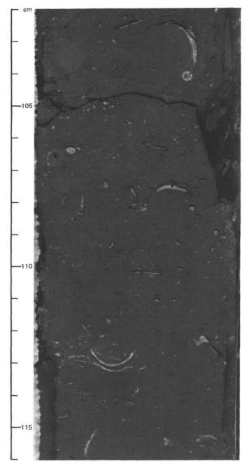
Figure 13. Skeletal olive gray chalk from Unit V, Section 627B-47X-5. Skeletal debris includes oyster valves and echinoid spines.
