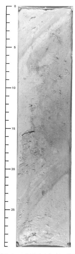
Figure 8. Carbonate oozes with inclined laminations interpreted as slump, Section 627B-6H-7.
