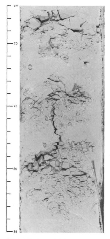
Figure 12. Chalk/ooze sequences in Unit III. Chalk is highly fractured; ooze may be drilling paste. Section 627B-27X-3.
