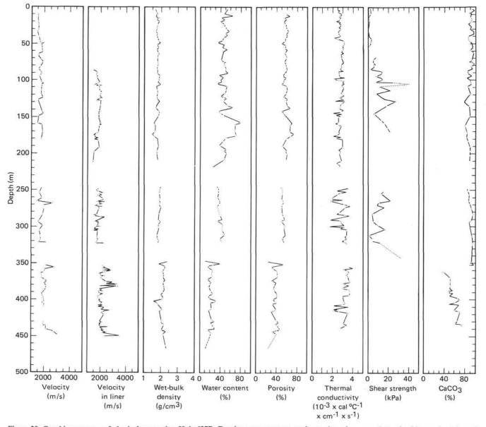
Figure 30. Graphic summary of physical properties, Hole 627B. Density, water content, and porosity values were determined by gravimetric and volumetric techniques.
