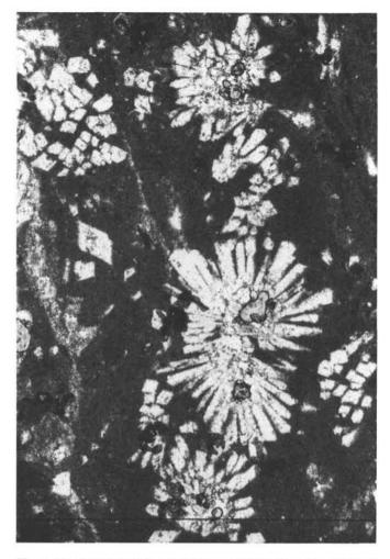
Figure 16. Thin-section photomicrograph of dolostone-gypsum facies of Unit VI. Note finely crystalline dolomite (dark) and replacement by radial crystals of gypsum (light). Small euhedral rhombs of dolomite are also present. Crossed nicols; long dimension of photomicrograph covers 32 mm.
