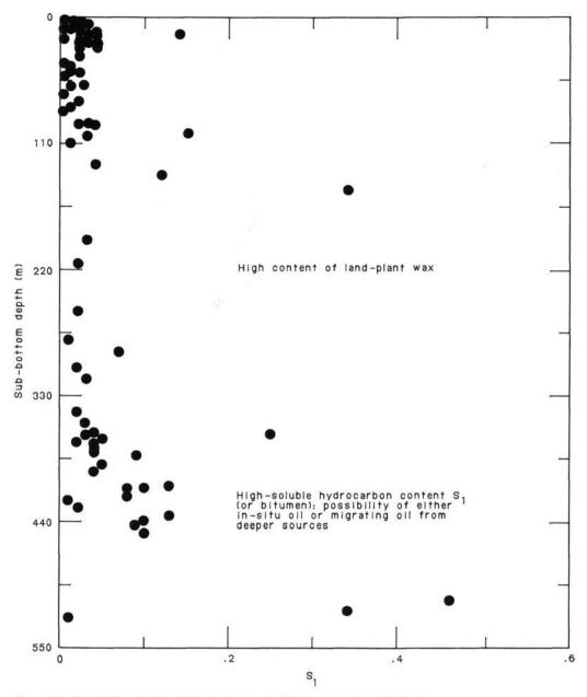
Figure 25. Downhole variation in bitumen content (soluble organics), Hole 627B.
