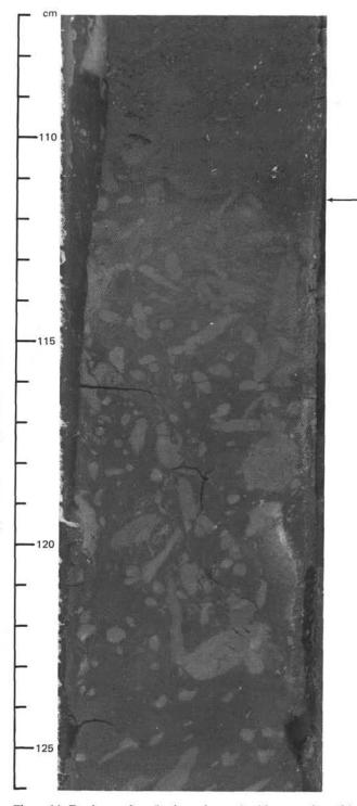
Figure 14. Erosion surface (horizontal arrow) with truncation of burrows. Unit V, Section 627B-39X-2.
