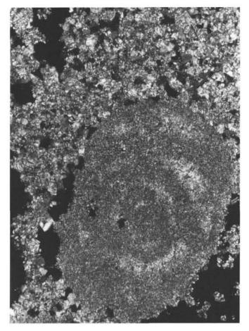
Figure 17. Thin-section photomicrograph of dolomitized miliolid from Unit VI. Larger subhedral dolomite crystals adjoin voids (black). Crossed nicols; long dimension of photomicrograph is 32 mm.
