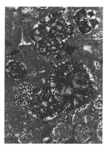
Figure 11. Thin-section photomicrograph of silicified limestone in Unit II. Note planktonic foraminifers infilled and partly replaced by chert. Planktonic foraminiferal packstone. Crossed nicols. Long dimension of photomicrograph covers 8 mm.
