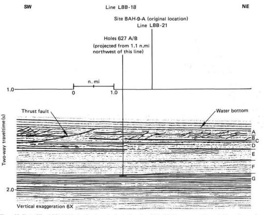
Figure 33. Part of line LBB-18, illustrating the seismic stratigraphy of Site 627. Sequences A through G are discussed in the text. The vertical line denotes depth of penetration of Holes 627A and 627B. Note the thrust faults displacing the section, particularly the large one landward (southwest) of Site 627.
