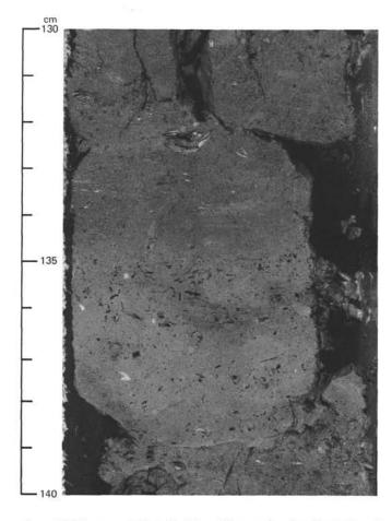
Figure 15. Limestone in Unit V with moldic porosity after dissolution of bivalve fragments, Section 627B-47X-6.
