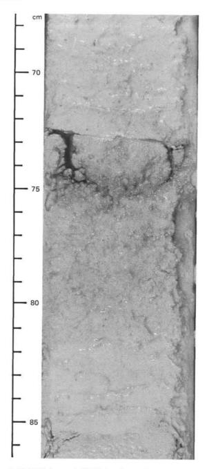
Figure 7. Unlithified to partly lithified packstone, interpreted as a turbidite, with lithification at the top of the turbidite, Section 627B-9H-5.
