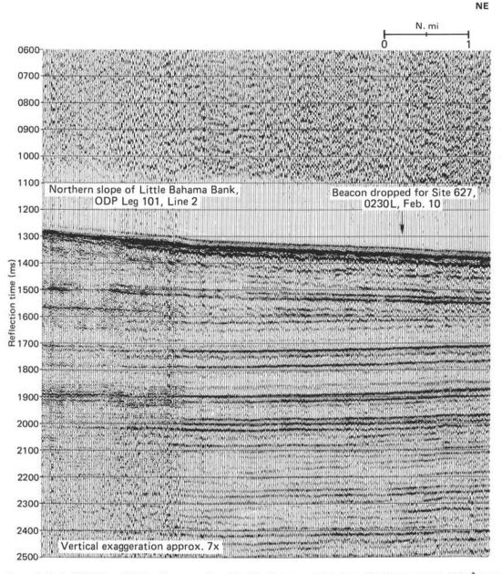
Figure 5. Part of ODP Leg 101, line 2, approaching Site 627. Data sampled at 1 ms. Sound source: two 80-in.<sup>3</sup> water guns, rep. rate 12 s. Leader length: 400 m.
