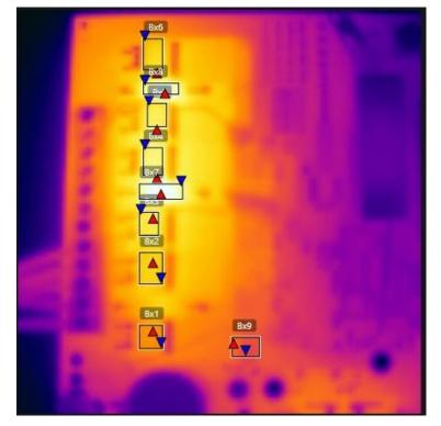
Figure 7: Thermal camera picture at end of current rating test
