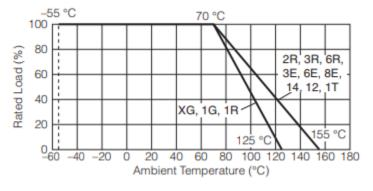
Figure 16: ERJ series chip resistor, power derating
