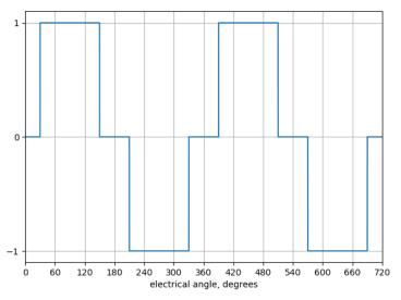
Figure 18: Typical six-step current waveform
