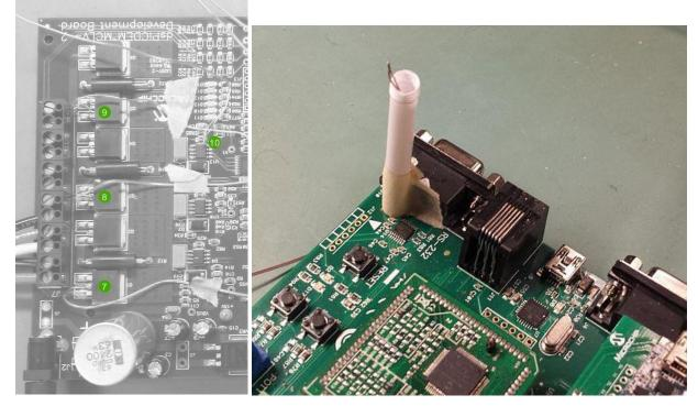
**Figure 5: Thermocouple setup**. Items shown in left picture are (7), (8), (9): type T thermocouples soldered to drain pins of Q1, Q3, Q5, and in right picture is a fourth type T thermocouple measuring ambient temperature near the MCLV-2 board.
