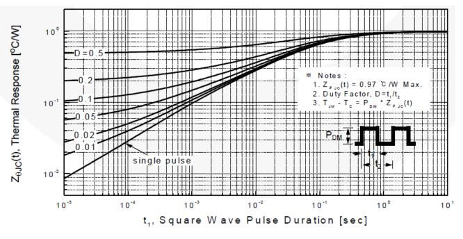
Figure 9: ON Semiconductor FQB55N10 transient thermal response curve graph (Figure 11 from datasheet)
