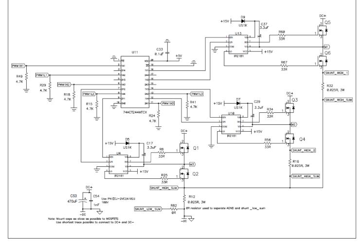
Figure 13: MCLV-2 components affected by Vdc (excerpt from the dsPICDEM™ MCLV-2 Development Board User's Guide, DS52080A page 34)
