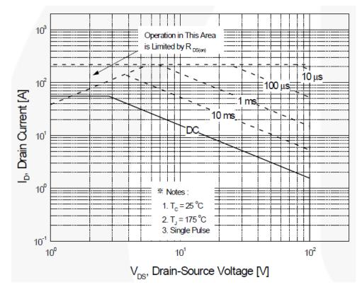
Figure 8: ON Semiconductor FQB55N10 single-pulse safe operating area graph (Figure 9 from datasheet)
