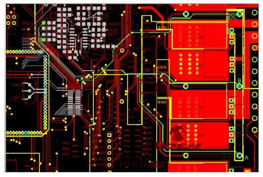
Figure 21: MCLV-2 current sense layout error
