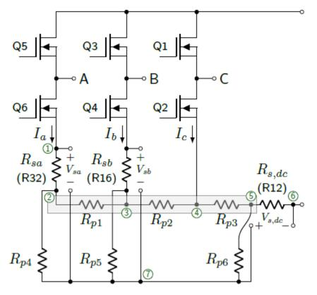
Figure 22: MCLV-2 current sense layout error (schematic equivalent)
