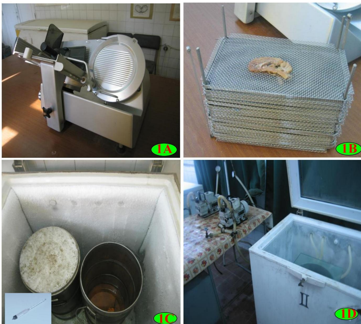
Figure 1. P40 room in Plastination Laboratory, Zagazig University. A: Rotary meat slicer used in sheet brain plastination for cutting the latter fixed brain during P40 technique, blade diameter: 210mm: rotate speed: 8000 round/min (adjustable). Slice thickness adjustment: 4 mm; B: Stainless steel grids as a carrier of brain slices; C: Freezer containing two dehydration acetone panels and an acetometer using in the step of dehydration of the latter fixed slices and D: Freezer containing P40 filled kettle which connects with vacuum pump and a monitor using in the step of forced impregnation of the latter dehydrated slices.
