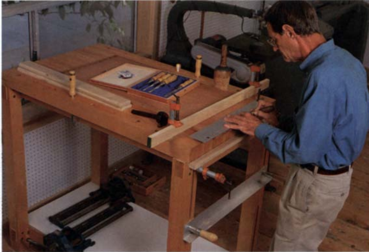
Marking tails —The author uses an aluminum template to mark out the tails on the side board of what will be a mahogany blanket chest. The short sections of pipe clamp at the front of the dovetailer's bench ensure the board remains flat for an accurate layout.
