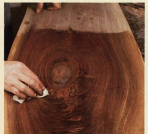
Step C: Oiling the wood reveals the colors of the repaired areas. Darkening the fillers with dye will finish them to a near perfect match of the knot.
