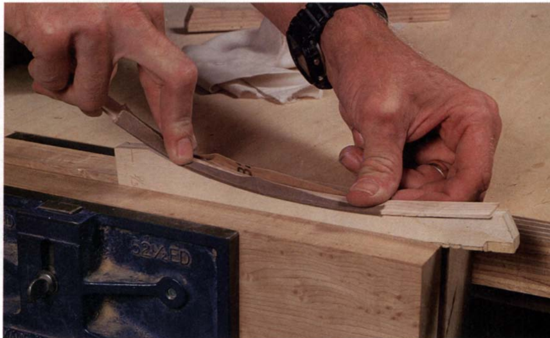
Shaping corbels —The author takes down the high spots on the corbel template's jigsawn curve with sandpaper backed by a flexible stick (above).
