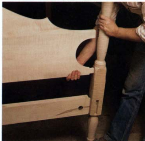
Assembling the head of the bed —After Latta loosely tightens the bed bolts between the head rail and posts (bottom), he checks the fit of the headboard.
