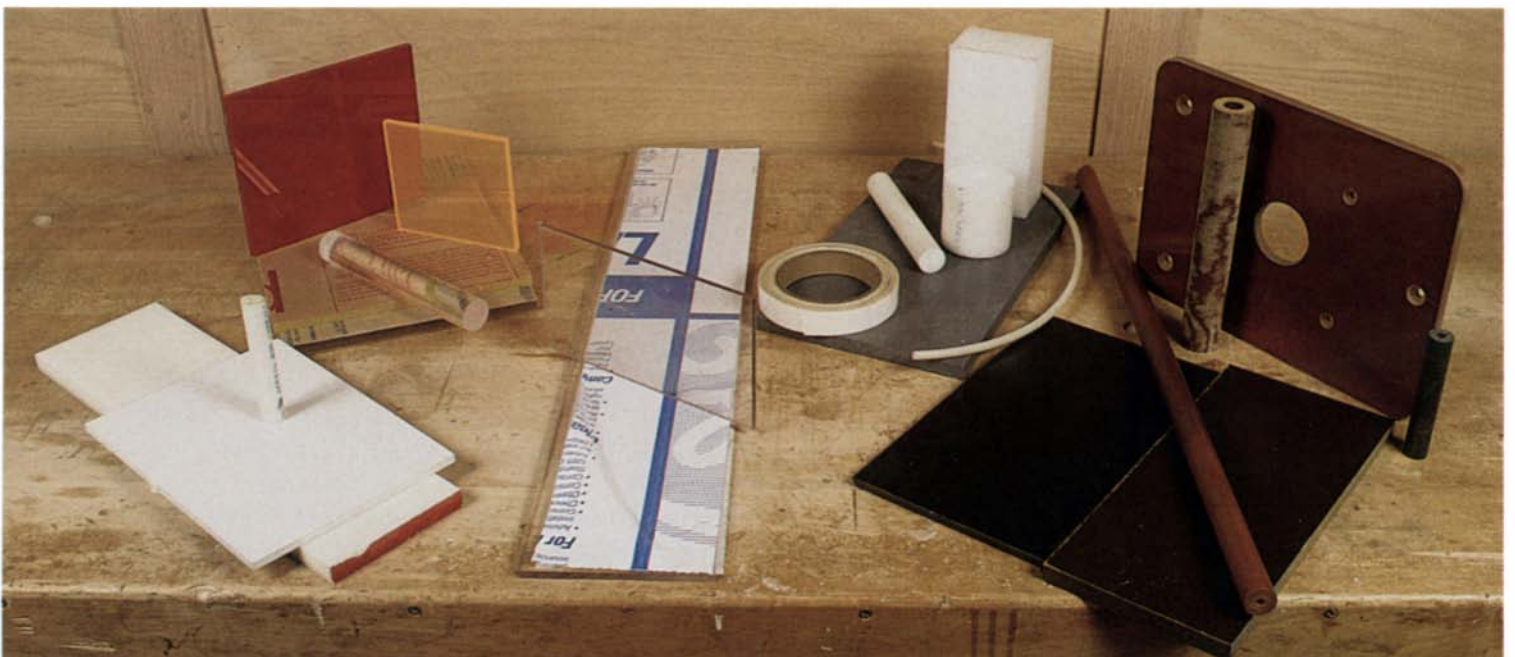
A myriad of plastics helps woodworkers make better jigs, fixtures and shop-built tools. From left: Slippery acetals make good bearing surfaces; rigid and clear acrylics are handy for templates; the impact resistance of polycarbonates protects you as machine guards; polyethylenes are tough and slick and great for sliding parts; and rigid and strong phenolics have no peer for table-mounting routers.
