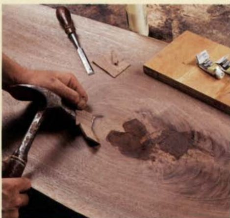
Step A: Filling the knot involves spreading a mix of epoxy and sawdust into the cracks and then driving and gluing in shaped wedges into the gaps.
