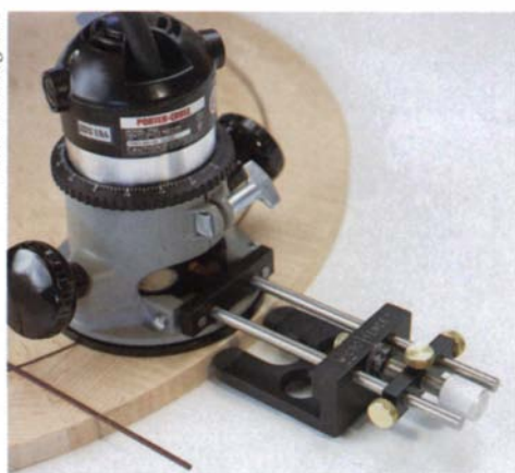
A precisely adjustable router fence, the Micro-Fence allows for accurate routing of odd-sized rabbets, dados and other precision cuts. It's a great accessory for dealing with undersized plywood, routing grooves for inlay, as shown here, or for fine-tuning the depth of a hinge mortise.
