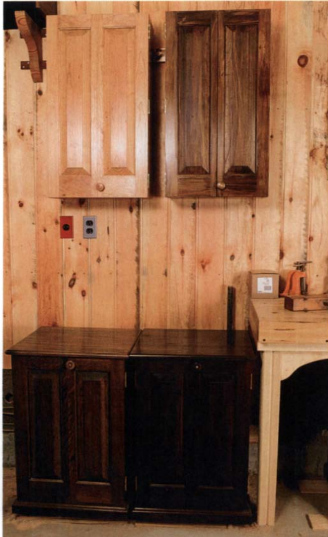
These movable cabinets keep tools stored, on slide out shelves or in drawers, neat and dust-free. Casters make the base cabinets mobile while a cleat-mounting system allows the wall cabinets to be easily rearranged.
