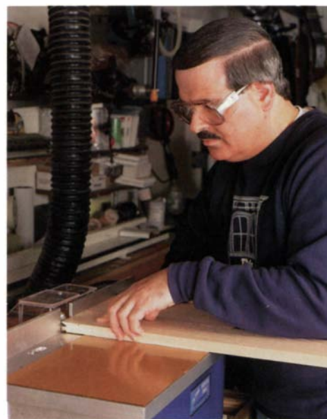
Versatile router table —CFW Engineering's new tilt-top router table allows you to create different molding profiles by varying bit angle and depth. The table also permits horizontal router mounting.
