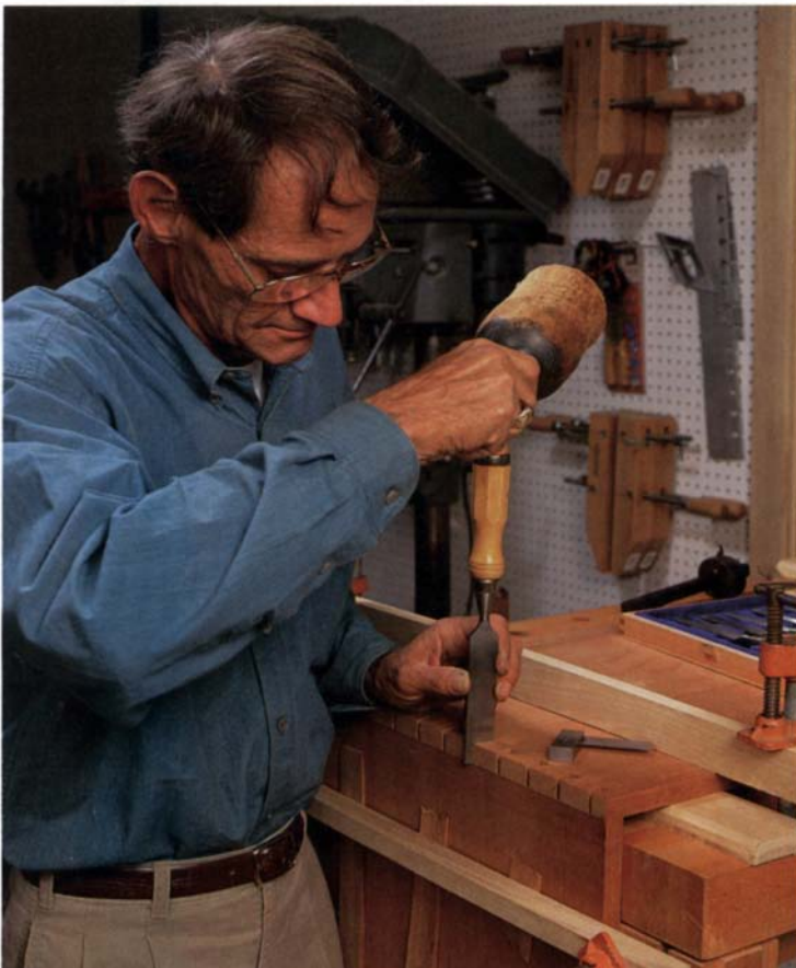
Marking pins from tails is more certain with a chisel than with a knife because there's no danger of the chisel following the grain. It's important, though, to make sure the chisel is absolutely perpendicular to the surface of the board you're dovetailing.
