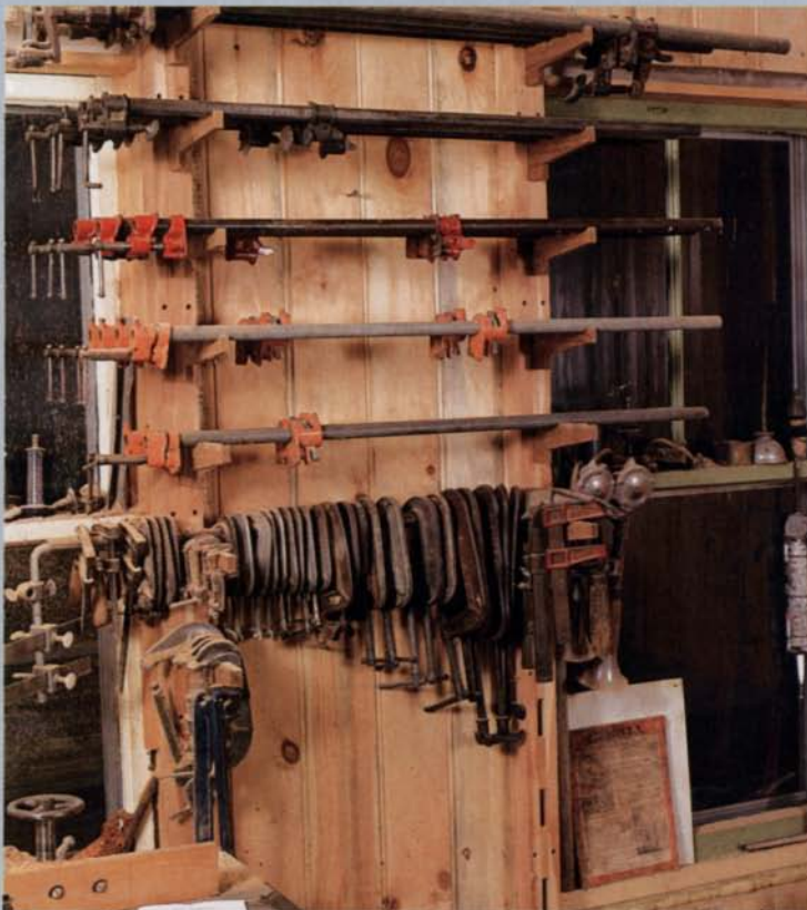
Wall racks for clamps and lumber storage are easily made by sandwiching spacer blocks between a pair of vertical supports. Support arms slide into mortises and are secured with a wedge.
