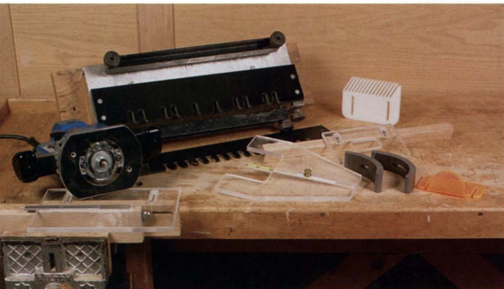
Plastics for jigs and fixtures —A shop full of accessories can be built with plastics. Clockwise from the bench vise: a mortise jig, a router subbase, a dovetail fixture, a featherboard, a hinge jig, a router-bit guard, hold-down clamps and a router-bit setting gauge.
