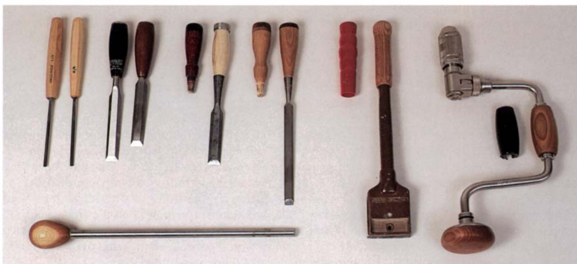
Rehandling a shopful of tools —Shown here are before (on the left) and after examples of tools that have modified or new handles. From the left, Pfeil carving gouges (edges eased and sanded), Stanley #40 chisels (handle replaced, new steel cap), Stanley #750 socket chisels (handle replaced, stainless steel hoop), Greenlee chisel (handle reshaped), Allway Tools scraper (handle replaced), Stanley #923 brace (handles replaced), Shopmade lathe knock-out bar with black locust knob.
