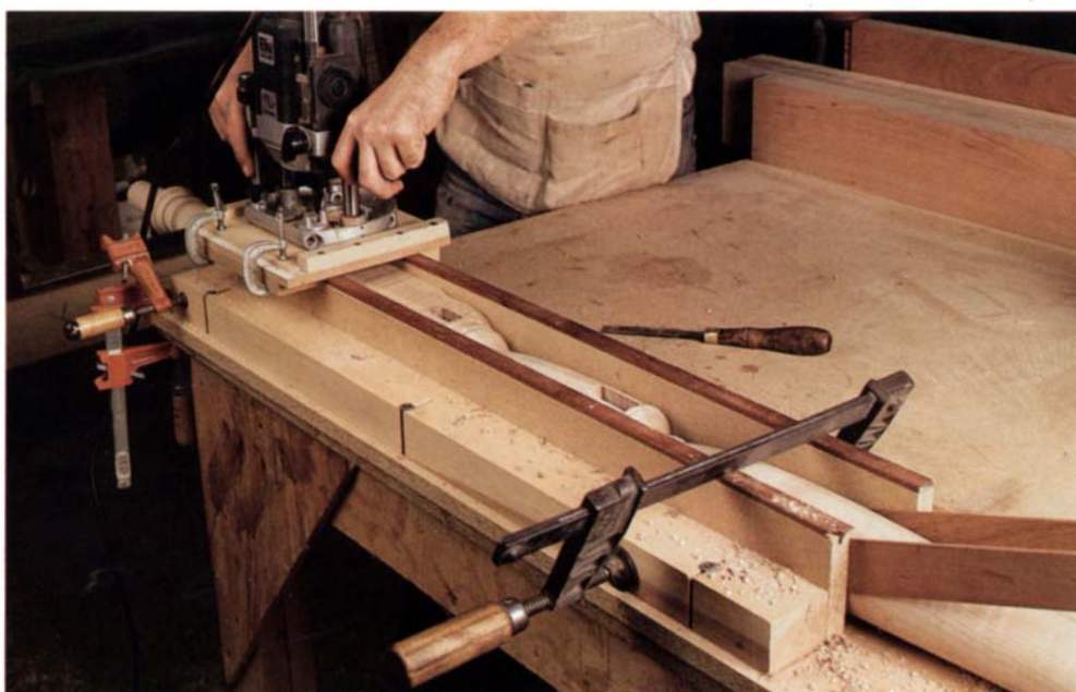
Routing bed-post mortises —With a post wedged in this jig, you can easily rout mortises for the rail tenons whether the post is turned or shaped. Then just use a chisel to square the mortises' corners. For adjustability, the router base slides in tracks in the carriage, and one of the jig's rails has slots for its mounting screws.
