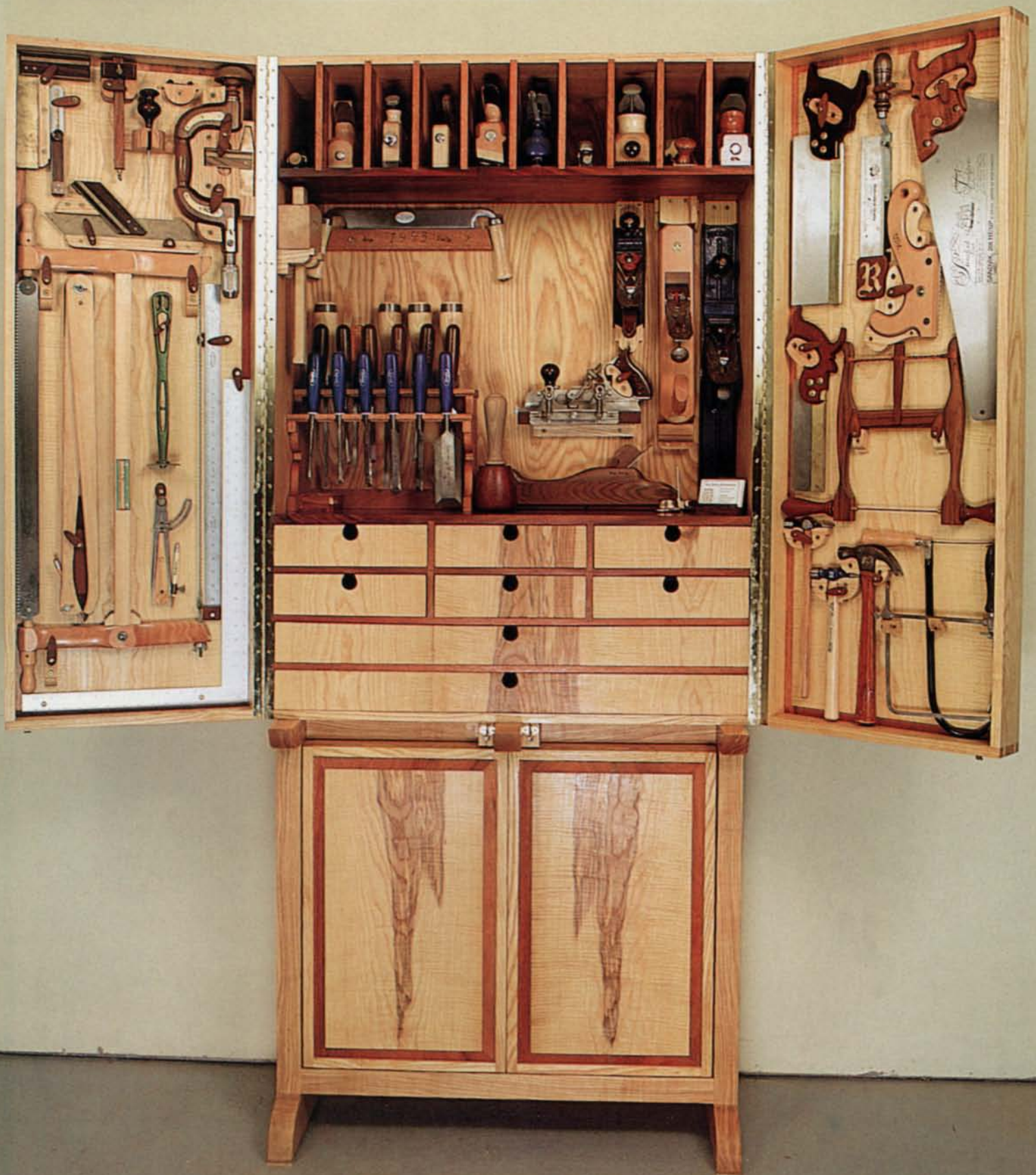
Being able to see his tools and get to them easily was a priority for furnituremaker Greg Radley of Ventura, Calif., when he started designing this tool chest. Radley's solution was this chest-on-trestle with a utility cabinet tucked into the trestle below. The trestle and all frame components are solid ash, the panels are solid mahogany veneered with curly European ash and the interior partitions are all mahogany.
