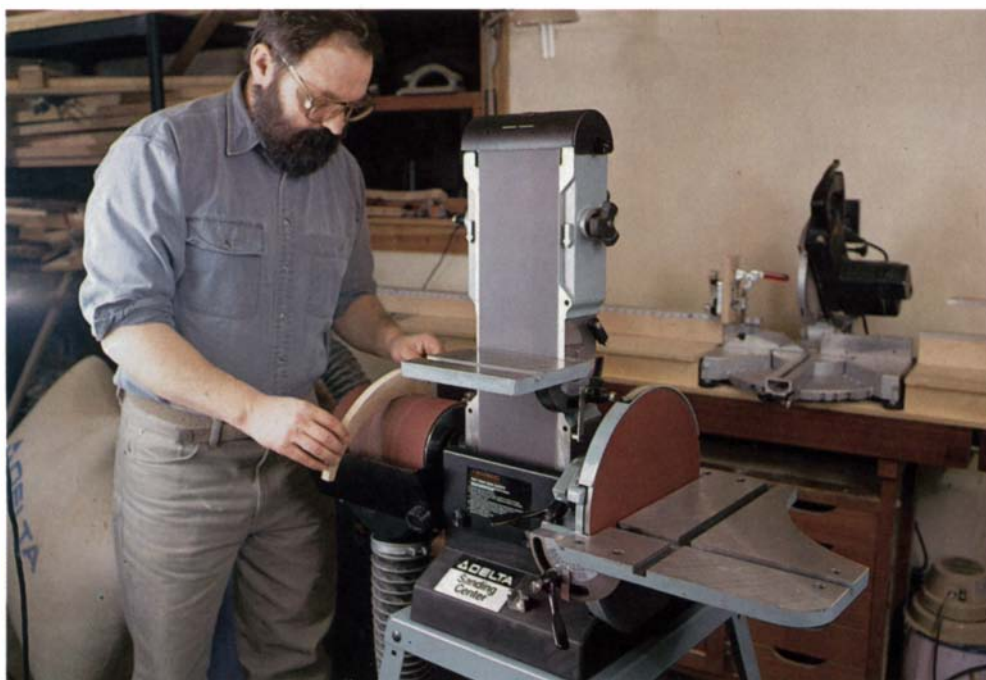
Three sanders in one —Delta's Sanding Center puts stationary belt, disc and pneumatic drum sanders in one station. A heavy-duty 1½-hp motor powers the unit.
