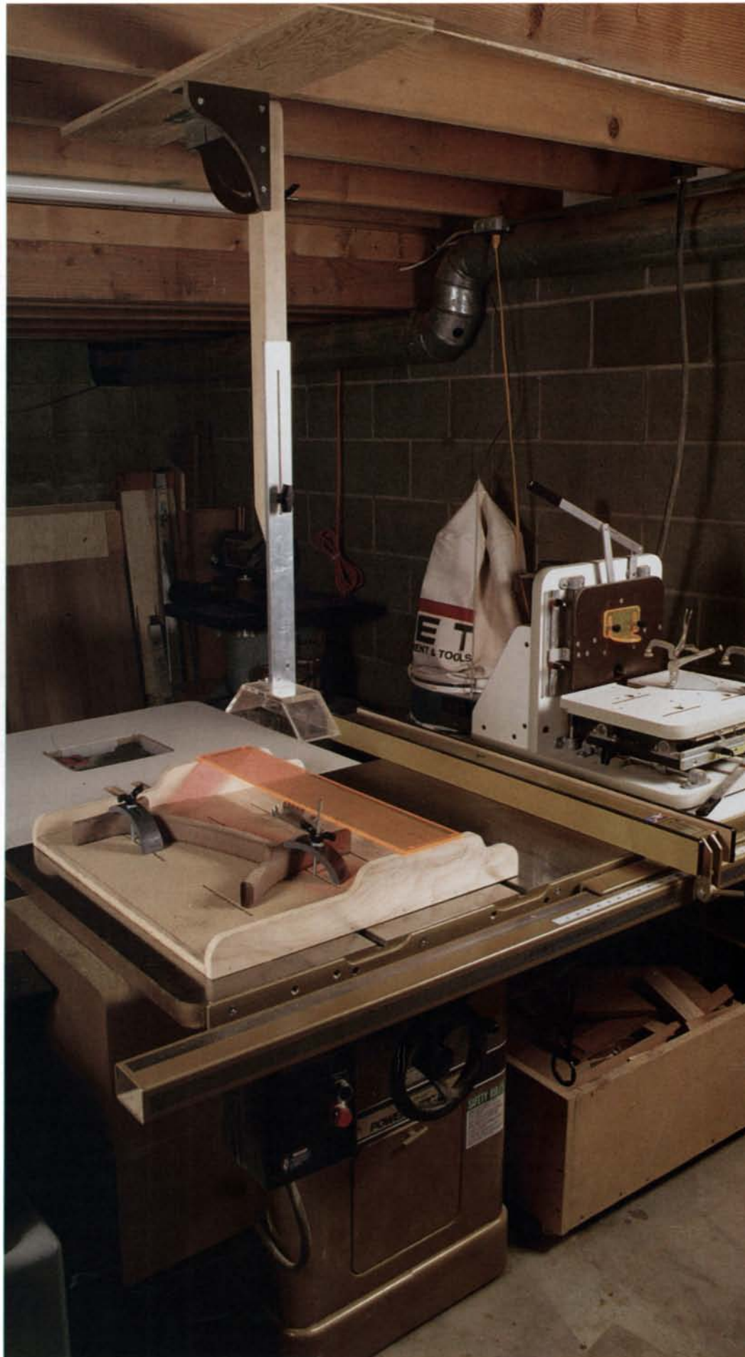
Plastics in the shop —Although this is a woodworking shop, plastics play a vital role, from holding workpieces in place, guarding cutting tools and guiding crosscut boxes to mounting routers and providing work surfaces. No shop would be complete without these handy materials that can make your shop-built tools more professional.
