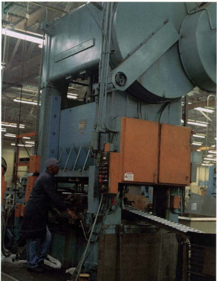
A 300-ton punch press is a deafening behemoth capable of stamping out one machine's sides every couple of seconds. With one motion, the machine can sever rolled-steel stock, form it around removable fixturing, punch holes in it and create louvers.
