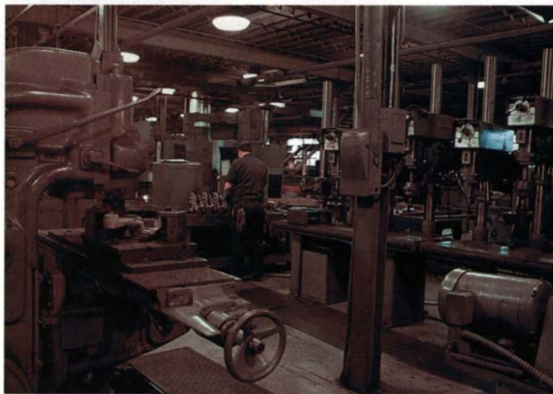
Powermatic still relies primarily on traditional machinery dedicated to single tasks as part of each work cell, though its manufacturing process has changed completely. Even so, with power feeds on much of the equipment, operators can move parts through several operations at the same time in a cell.
