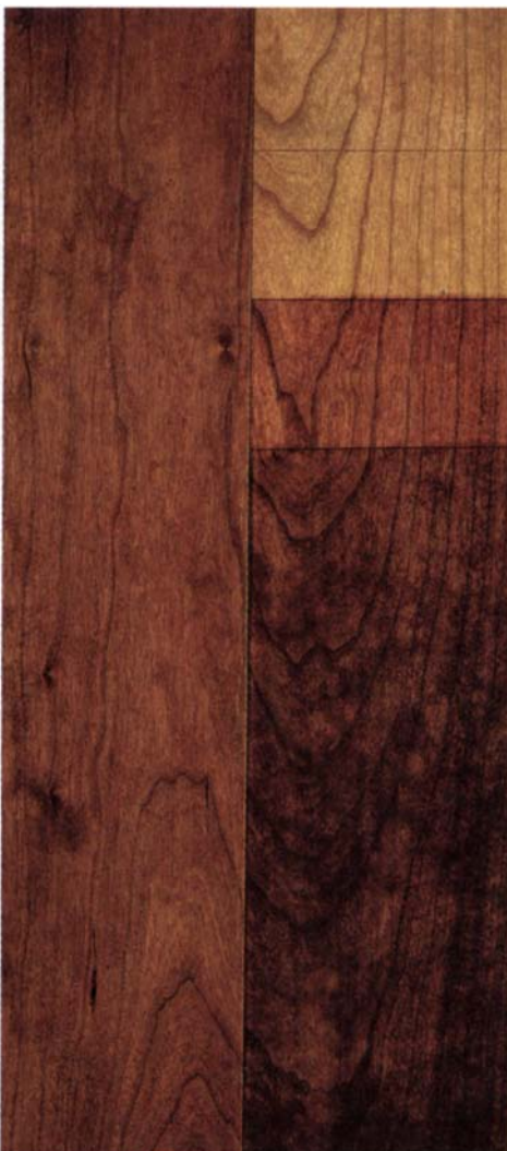
Stains can be mixed or applied in layers. Solvent-compatible stains can be mixed together in the can and applied at once, here over cherry (left sample). Note the difference in the right sample showing the same three stains applied one at a time (from top to bottom): unstained cherry, yellow, reddish mahogany and medium-brown dye stains.
