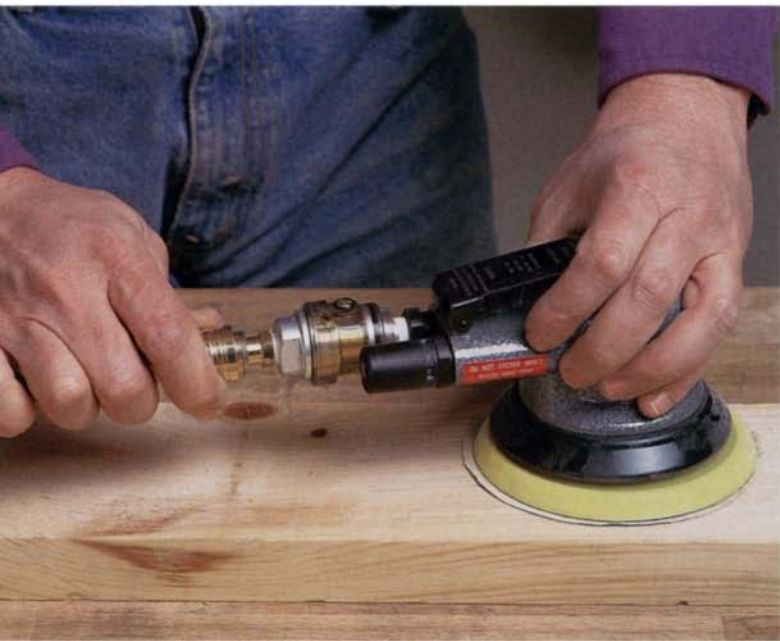
An air-tool oiler automatically lubricates an air sander as the tool is used. A muffler on the Dynabrade sander shown here (the black cylinder in front of the oiler) reduces air exhaust noise.
