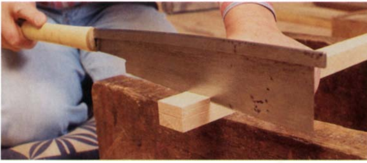
The rigid-backed dozuki-noko makes fine crosscuts with small teeth that leave a very smooth cut surface. It's a good choice for cutting tenon cheeks, as shown here, or for other joinery.
