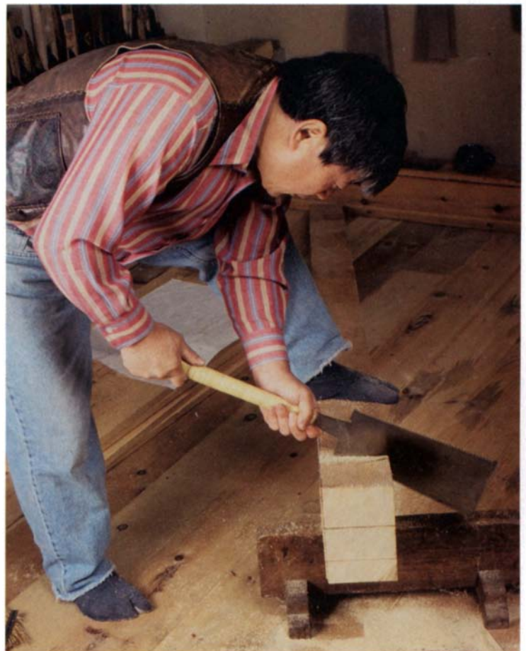
Using two hands on the ryoba-noko yields maximum power and control. Here the author cuts a tenon's shoulder, using the saw's crosscutting teeth. He'll flip the saw over and use the rip teeth on the other edge for cutting the tenon's cheeks.
