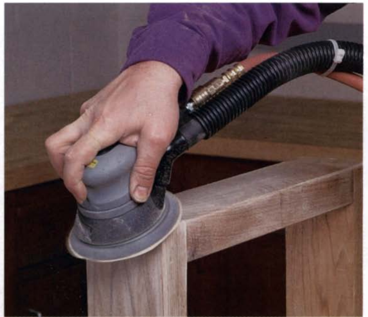
A venturi driven by exhaust air collects sawdust on the Sioux 690VV. The air propels the dust down a flexible hose (fastened to the air line) into a canvas bag.
