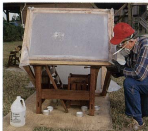
Using 26% ammonia to fume the wood gives distinctive color, but rubber gloves, protective eyewear and breathing apparatus are a must. Cups of ammonia are placed inside the plastic-sheet fuming tent with items to be fumed and left overnight.
