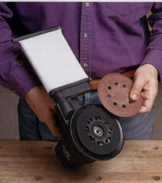
The Porter-Cable 332's porous-plastic canister collects sawdust, just like a regular canvas bag. The small container easily dismounts for emptying.
