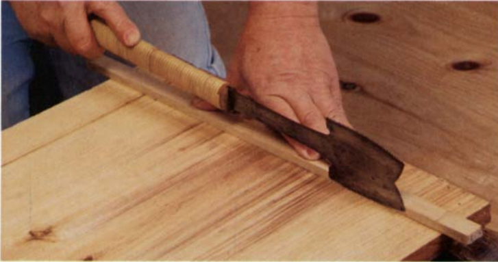
The azebiki-noko can start a cut in the middle of any surface, allowing it to do cutouts or stopped grooves. The author uses a straight stick to guide the saw while cutting the sides of a slot, which will be chiseled out later.
