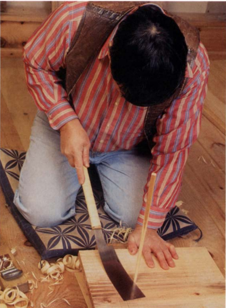
A kugihiki-noko can flush trim a dowel and leave behind a smoothly cut surface that needs no further sanding. Its teeth have no set, so they won't scratch the surrounding panel.
