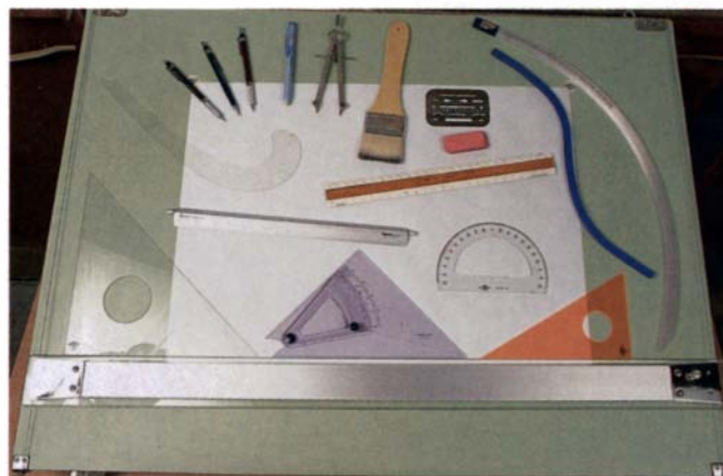
Drawing supplies used by the author include, clockwise from lower left, a 45° to 45° angle template, a metal architect’s rule, a ship’s curve (a large version of a French curve), mechanical pencils in three sizes (3mm, 5mm and 7mm), a pencil-style eraser, a compass, a dust brush, an eraser shield, a pink eraser, a flat architect’s rule, a lead flexible curve, a plastic adjustable curve, an orange 30° to 60° angle template, a protractor and an adjustable angle template.
