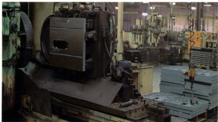
Surfacing saw and shaper tables is a two-step operation. The tables are first taken down to within .020 in. of flat and are later ground to .005 in. or less depending on the table. The hoist on the right is used to move the tables.
