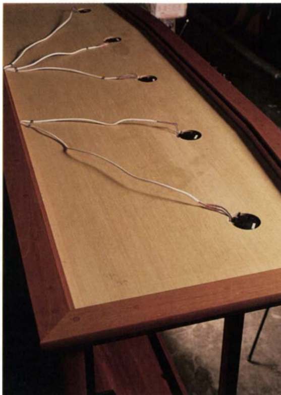
Down lighting —Dan Trimble of Indiana, Penn., custom-made this cabinet to house a collector's rifles. To ensure the guns would be well lit, Trimble installed five, 12v, 20-watt halogen spotlights overhead. The battens in the back will be covered by mirrors.
