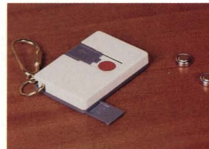
Lighting controls —The gun-cabinet lights (above) can be controlled with this pocket-sized remote unit or by a switch in one of the drawers. A cavity in the lower case houses the low-voltage transformer and the remote's transmitter.
