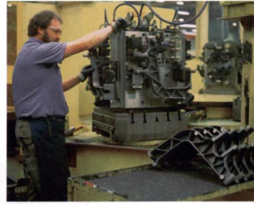
Hydraulic fixturing and independently programmable cutterheads make computerized machining versatile (above). Here, a worker adjusts the clamping pressure on a rough casting.
