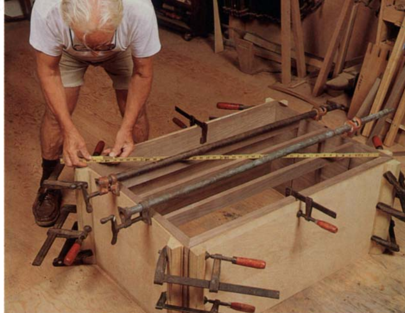
Above: To check the carcase for square, Frid measures across the diagonals. He placed the thin-plywood assembly jigs on the outside of the carcase. The jigs are the same size as each carcase piece, with beveled cleats on each end. Below: After routing the convex shape on a drawer front, Frid rips a 20° bevel in its top and bottom edges so the front's edges are straight and flush with the straight carcase front.
