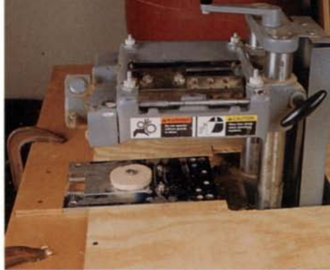
For molding curved trim, the author uses an auxiliary table with two small bearings mounted about 2 in. apart. A guide groove routed into the back of the trim piece rides on the bearings and holds the trim in proper relation to the cutter.
