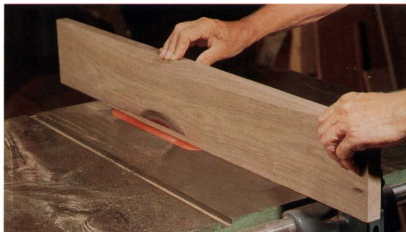
Above: To check the carcase for square, Frid measures across the diagonals. He placed the thin-plywood assembly jigs on the outside of the carcase. The jigs are the same size as each carcase piece, with beveled cleats on each end. Below: After routing the convex shape on a drawer front, Frid rips a 20° bevel in its top and bottom edges so the front's edges are straight and flush with the straight carcase front.
