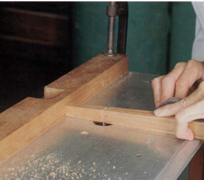
The author routs the banding groove in a leg by running the miter gauge bar along the router table's front edge. The router-table fence, which locates the cut, is clamped parallel to the table's front edge.
