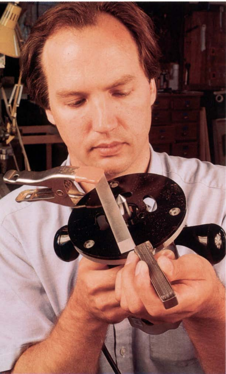
A simple method for determining the concentricity of the collet employs a bar clamped to the base and a special pointed bit called a "know bit" (demonstrated here by Brad Witt of Woodhaven). A feeler gauge indicates the amount of runout.
