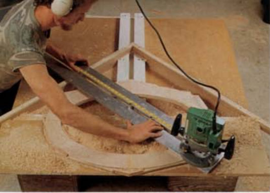
Schmidt designed his routing machine for cutting large ellipses. To cut out the small mirror frames, he added an auxiliary table to mount the frame atop the track and a right-angle bridge that supports the beam at the table's level.
