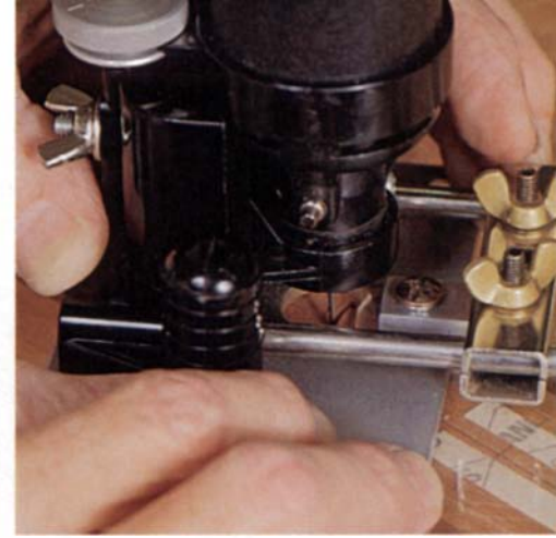
Left: Pittman uses a set of dividers with a dowel taped onto one leg to locate the plastic template for cutting the curved stringing grooves. Right: The arc is cut with a Dremel tool fitted with a screw that is inserted in one of the template's holes. The screw allows the bit to be pivoted through the \frac{3}{4} -in.-dia. arc.
