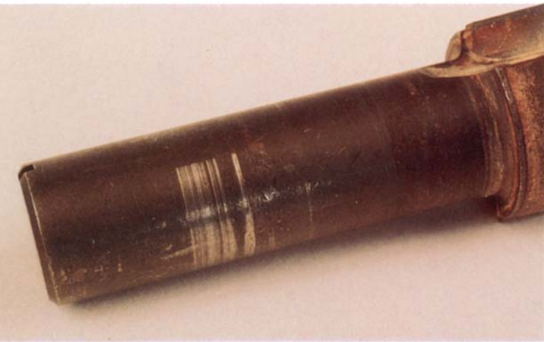
When a collet fails to keep a bit from slipping during a cut, galling can occur, which is shown here as the shallow grooves in the shaft of the bit. Fortunately, these can be filed off to restore the shaft.
