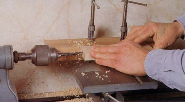
The author uses an auxiliary table on his lathe to end-drill the rails for reinforcing tenons. He drills these holes first, whether reinforcing tablesawn stub-tenon joints or shaper-cut joints.
