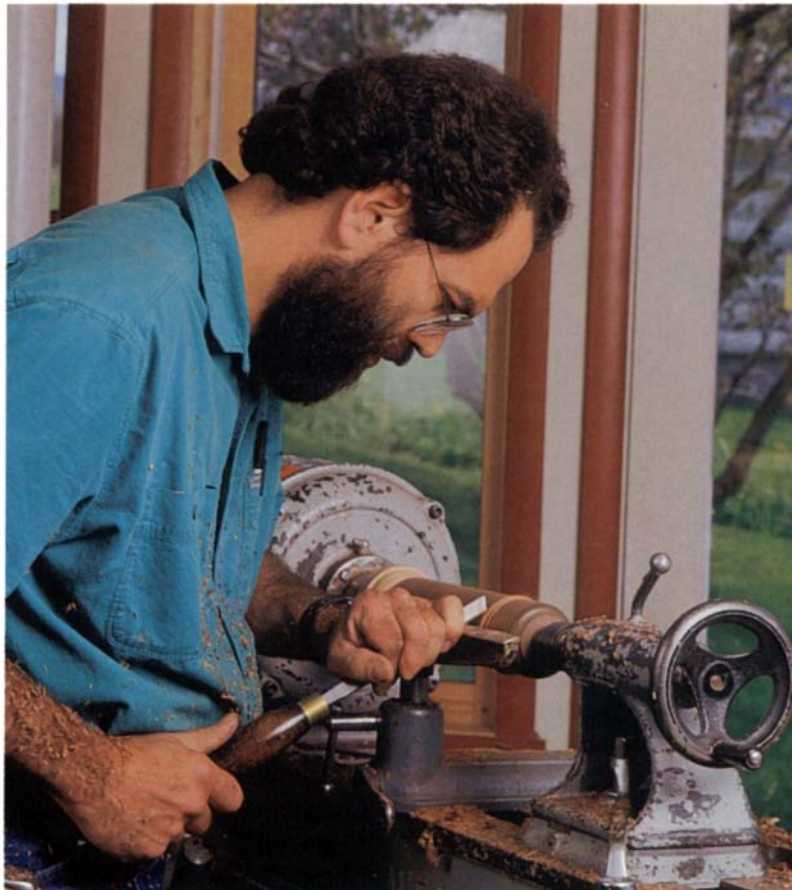
Gray pinches the glued-up barrel and eyepiece assembly between a ball bearing, cone center and a wood taper fastened to the lathe's faceplate. Then he turns the finished diameter, the object case tenon and decorations.
