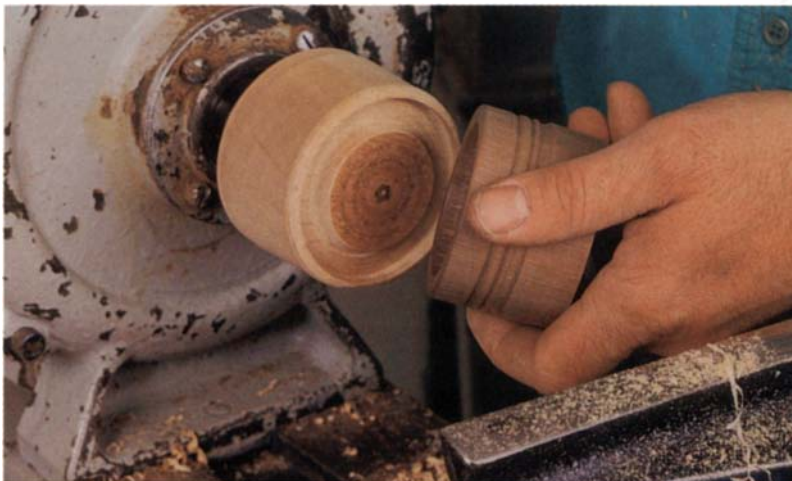
After turning the object case mortise, Gray cuts the case from the glue block. He then turns a groove in it, making the block a jam chuck to hold the case's lips so he can turn its other end.
