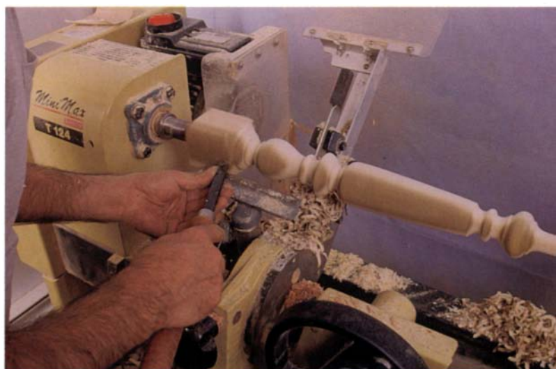
Above: This lathe was modified with a tool rest so the operator could easily crank the carriage into position to add hand-turned details, such as square shoulders and undercuts, which aren't possible with most semi-automatic duplicators. Below: Cutters come in a variety of shapes and materials; top row, left to right: mild-steel scraper, two HSS scrapers, carbide-tip scraper. Bottom row, left to right: tri-pointed HSS shear cutter, HSS reversible shear cutter, HSS shear cutter, and V-shaped HSS shear cutter.
