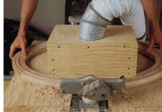
A frame blank, screwed to a plywood template that is grooved to ride on the guide bearings, slowly rotates through the molder. The spring-loaded wood disc presses against the template edge to keep it from shifting on the bearings.
