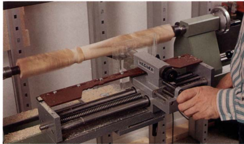
The spring-operated plunger mechanism of this semi-automatic duplicator pulls the stylus to the template and the cutter into the blank at the same time. Slots in the template for mounting screws allow adjustments; ramps at the end of the template act as carriage stops.
