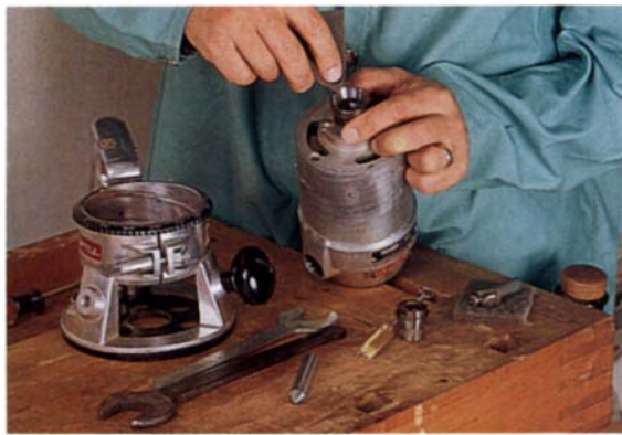
Cleaning your router's collet socket is a vital part of tuning this shop workhorse. Mark Duginske tells how on p. 56. Cover: Alec McCurdy's music cabinet blends tradition and uniqueness (article on p. 54). Photos above and cover by Sandor Nagyszalanczy.
