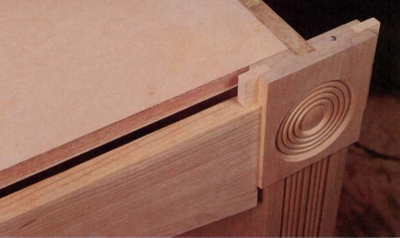
The cherry rosettes and valance strips that grace the top of the built-ins add a nice bit of visual detail to the otherwise simple upper cabinets. The parts are joined with loose maple splines fitted into grooves that Foster cut with a straight bit in the router table.
