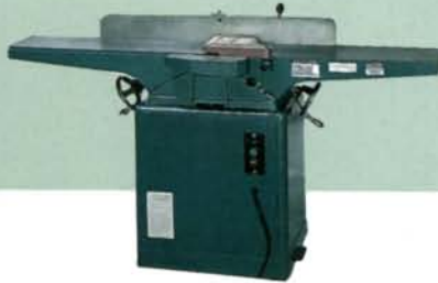
BW-8J JOINTER $869. Planes 8" wide and up to 1/2" deep rabbets. 3-knife cutter-head. 1 1/2 HP US motor. Other models from 6" to 16" wide.
