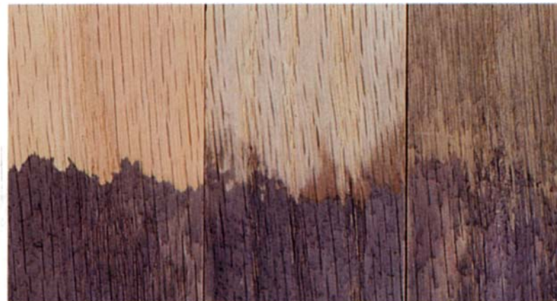
When bleaching iron stains from oak, oxalic acid virtually removes the blue-black stain from the sample (left), returning the wood to its natural color. A/B-type bleach (center sample) leaves the wood more silver, and chlorine bleach (right sample) leaves the wood gray.
