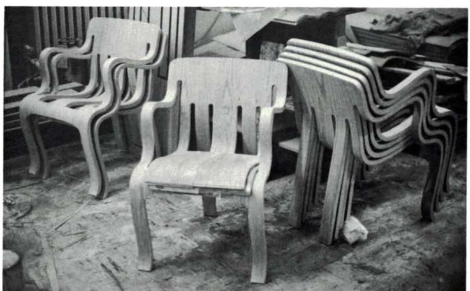
Either version of the one-piece plywood chair can be stacked for storage.
