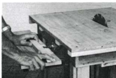
Horizontal mortising: Workpiece is pushed into bit and moved from side to side to clean out waste.
