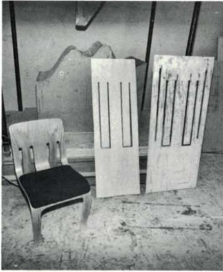
Peter Danko's one-piece plywood chair, left, is made from a 10-laminate sheet of slotted veneer, center. The pattern for routing the veneers for the chair with arms is at right.
