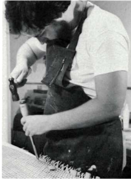
Trim cane ends by chiseling at outer edge of groove bottom.
