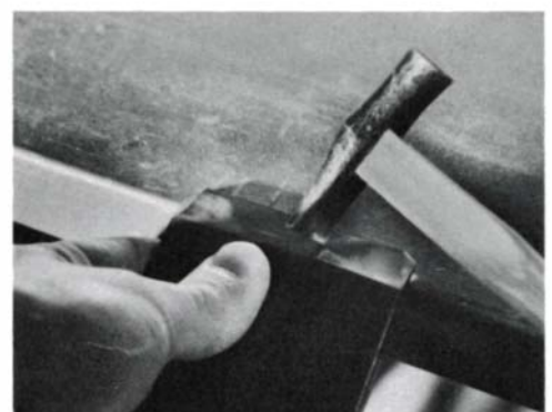
A kanaban, or iron board, sharpens the ura. A series of grinding powders pictured at top—kongosha, right (a sandstone grit), and second and third grinding-stone residues, center and left—are mixed with water on the kanaban and the blade ground back and forth over it to bring up a mirror finish. Bottom, because of the low-carbon steel in the blade laminate, the hollow ground on the ura can be pushed out by tapping the bevel on the omote with the pointed edge of a hammer while the blade rests on the corner of a hard metal surface. This is done when, after repeated sharpenings, the edge has been ground back into the ura hollow.
