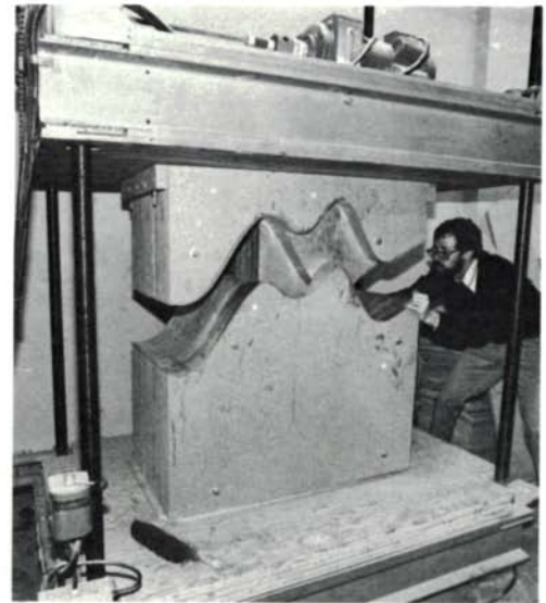
Danko opens the mold by bolting it to the upper platen of the press, built by George Danko to his son's specifications, and checks alignment as it moves up.
