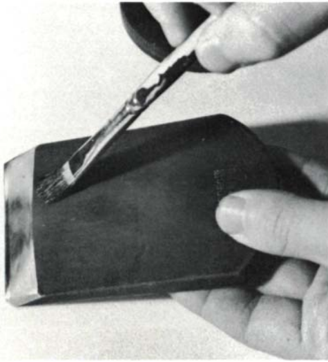
Paint the lower face and the two edges of the blade with ink, left, and while the ink is still wet, tap the blade in to register the high points in the groove. When the blade is tapped out, ink remains on the areas to be pared down, above.
