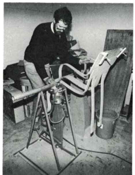
Danko runs jig over template router. Straight-flute bit protrudes through pipe; collar on pipe bears against jig.
