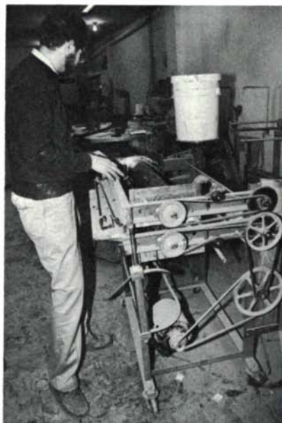
Glue-spreader coats both sides of the veneer in one pass. White bucket holds the glue; plywood guard normally covers pulleys.
