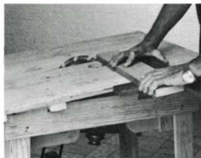
The crosscutting fixture consists of two crossed boards, glued and screwed at 90°. One board rides the edge of the table, the other pushes the work. A similar device permits 45° miter cuts.
