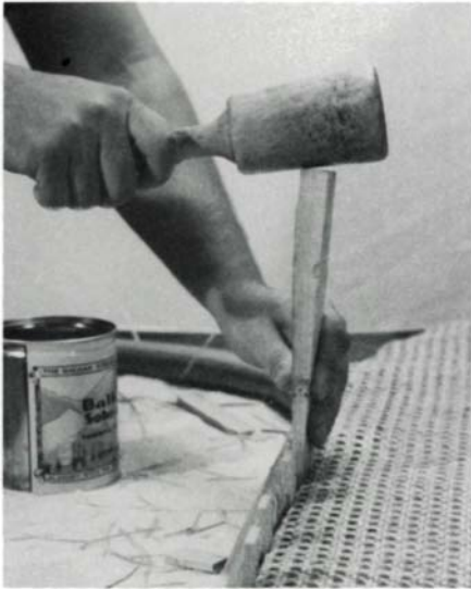
3. The cane is forced into the groove and held in place with a locking wedge.
