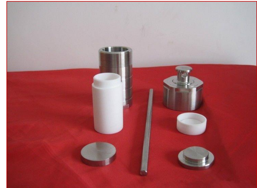
Hydrothermal reactor and the parts of the chamber
