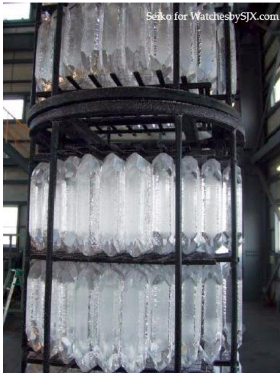
Hydrothermal grown synthetic quartz crystals. ( http://www.watchesbysjx.com/ )
