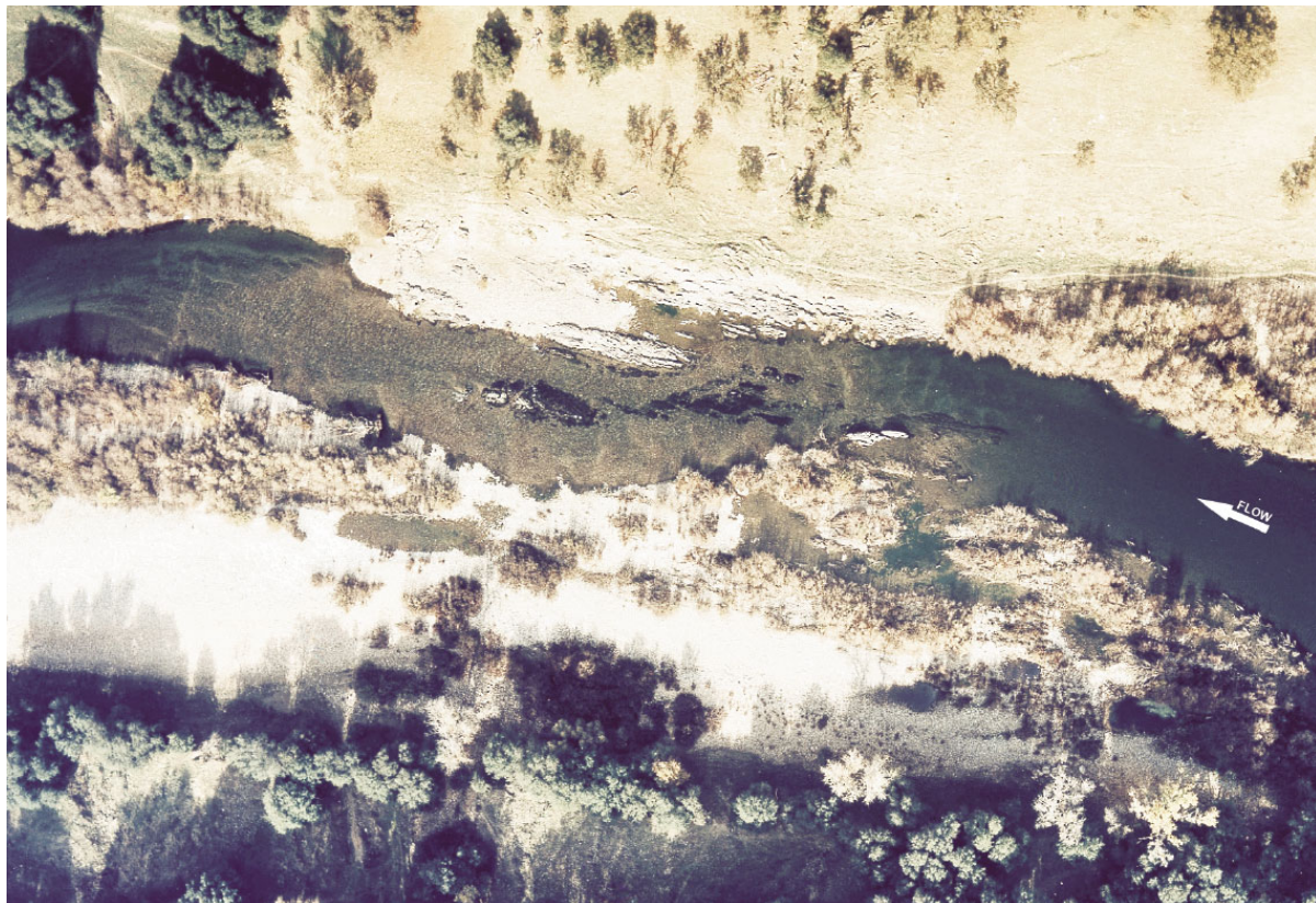
Figure 12. Aerial photograph from 1999 of Riffle A7 (RM 50.7). Successive floods and the lack of coarse sediment supply have slowly depleted the volume of coarse sediment stored in lateral bars.
