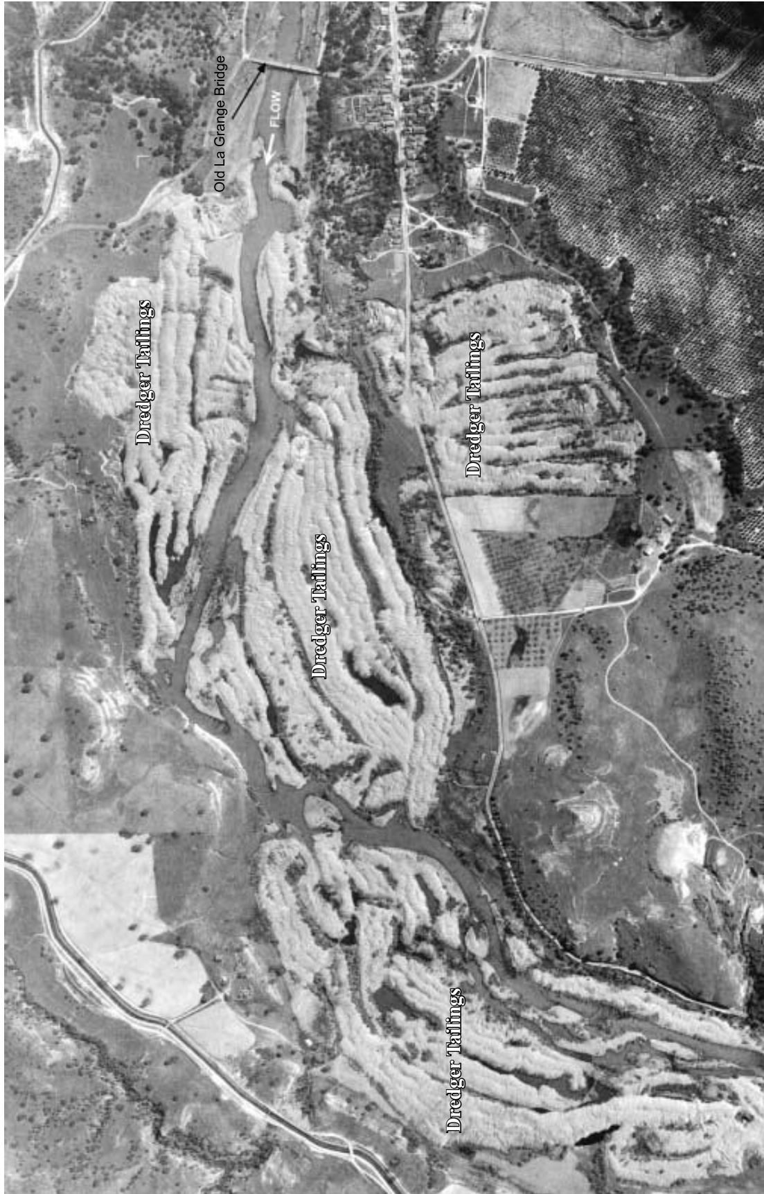
Figure 2. The lower Tuolumne River's dominant spawning reach from 1950 showing an example of the extent of gold dredging in the gravel-bedded reaches.
