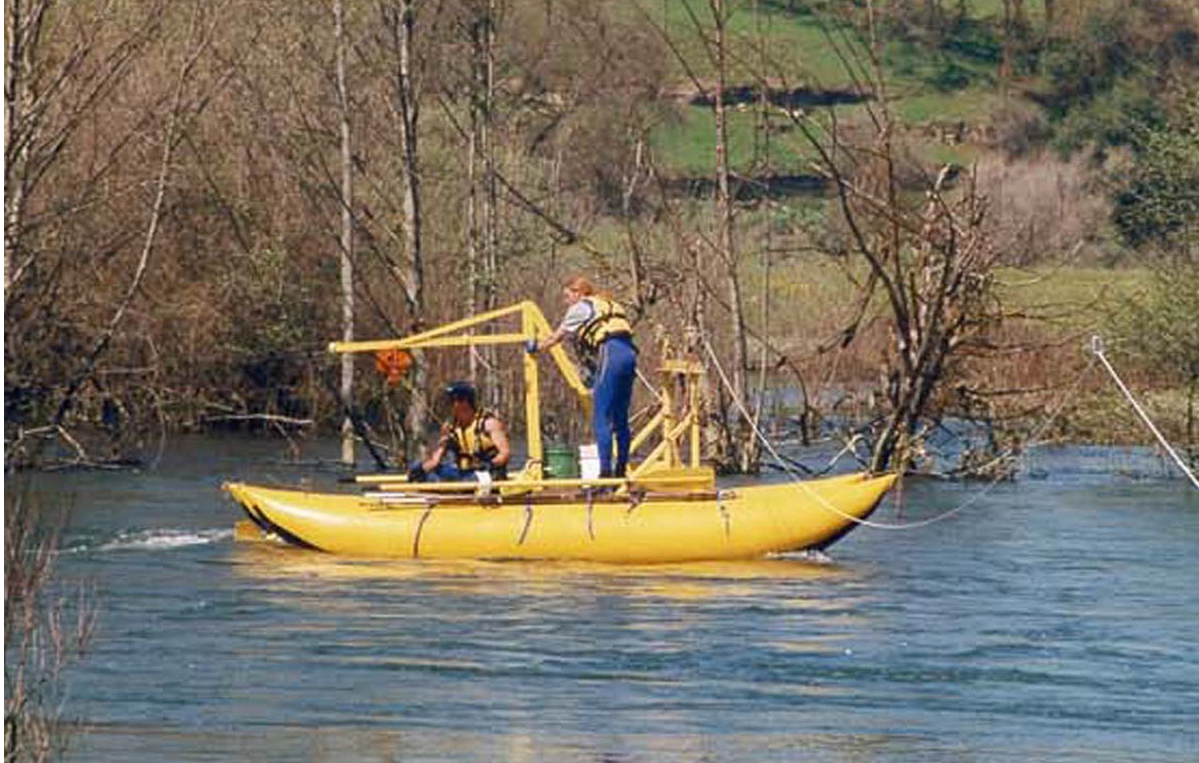
Figure 19. Bedload sampling at Riffle 4B on the Tuolumne River during a controlled flow release of 6,700 cfs. The Helley-Smith bedload sampler is lowered to the riverbed on the boom and collects sediment in transport for 60 seconds at multiple stations along the cross section.
