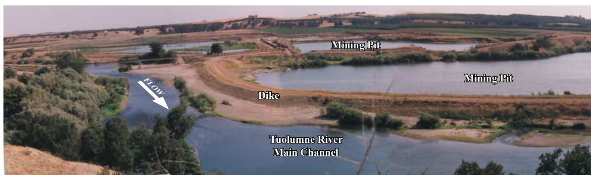
Figure 4. The Tuolumne River (in the foreground of photo) in the Gravel Mining Reach showing commercial aggregate mining operations near Waterford, which create huge floodplain pits adjacent to the low-water channel.
