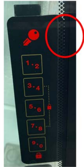
E: Light Leakage
