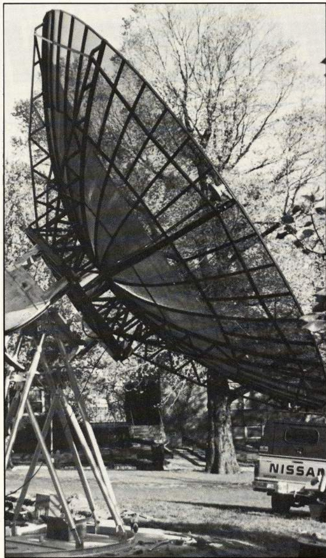
Polar mount with motorized Y axis created by Roundhouse for ECI 16 foot dish.
