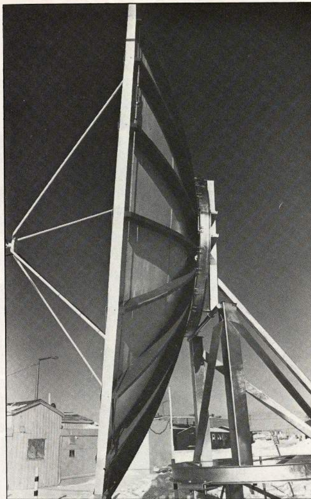
Straight line edge view of the 6.0 meter TVRO antenna indicates that all of its cross-sections share a common optical axis. The net result is a maximum concentration of satellite RF energy in a single focal point for high gain and low side lobes. This antenna employs a novel stressed/prestressed parabolic framework to ensure long-term shape-holding. Usage at low look angles causes some antennas to exhibit 'clamshell distortion' or petal droop. Photo courtesy of Paraframe Communications, Inc.
