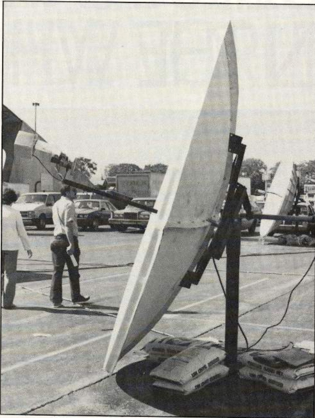
A severe case of 'rim wow.' This antenna's real world gain can only remotely approach its specified gain level. (Moral? Specs are merely ink on paper.)
