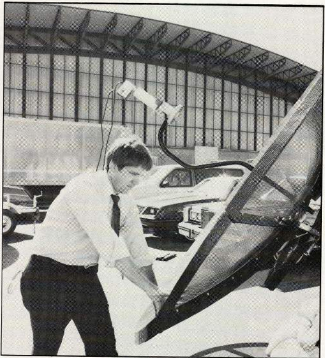
This aggressively advertised and promoted antenna's glaring design deficiency is the absence of an adequate rib backing structure to lock all of the ribs in the same plane (of revolution). Gently nudging a single rib set up a wave action around the entire dish circumference; not good for performance and definitely not good for long term survival in the elements.
