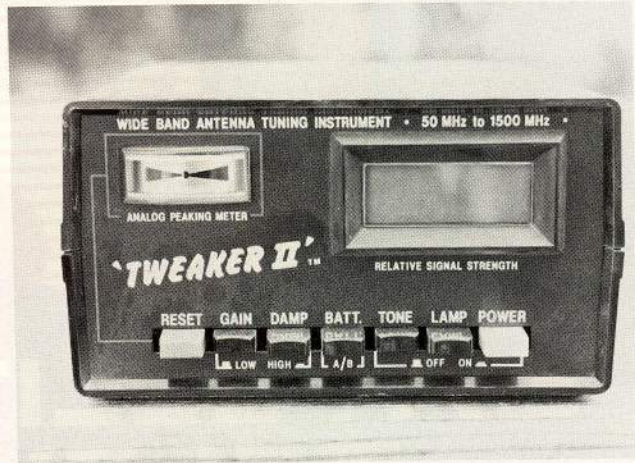
TWEAKER II front panel has row of buttons along bottom of case front to select metering functions.
