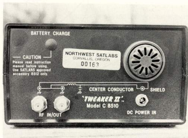
REAR PANEL of TWEAKER II includes a pair of 'F' style fittings; you loop-through the instrument and can power your LNA and downconverter with accessory 'power pack' unit (optional) for total wireless testing on a roof.
