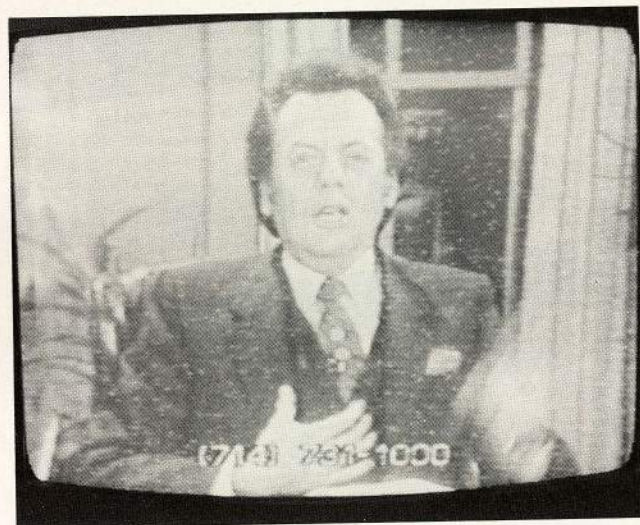
LOW END RESOLUTION TEST/ 'Weaker' (picture corresponds to meter reading, using strongest transponder from test dish)
