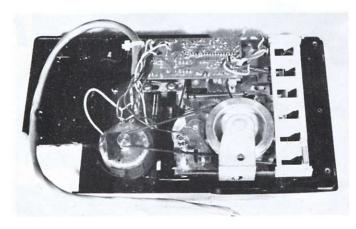
Photo 6. Gutted cassette is probably a stopgap measure. Note absence of usual electronics, speaker, jacks, etc.
