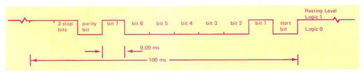
Fig. 2. The bit composition of the ASCII encoded character A (capital), and its associated timing values when transmitted at a rate of 110 baud. Note that the resting level is always logic 1, while the start bit is always logic 0.
