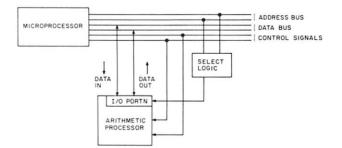
Fig. 1. An arithmetic processor in a microcomputer system.
