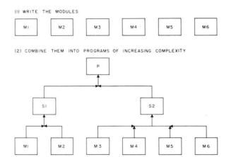
Fig. 1. The procedure for bottom-up design.
