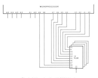
Fig. 1. Addressing the 1K RAM block.
