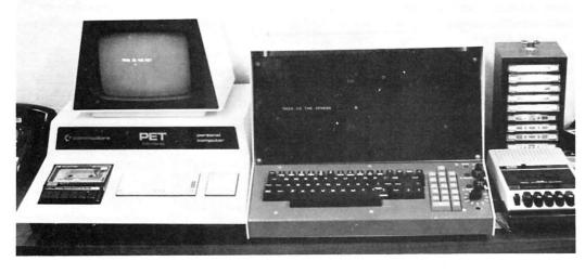
Photo 3. Now-defunct Sphere, right, is very similar to PET, left. Note the combined keyboard, TV, CPU, integral dual cassette controls and number pad. PET's cassette is built in.
