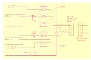
Fig. 1. The simple modifications to the Processor Technology 3P+S interface.
