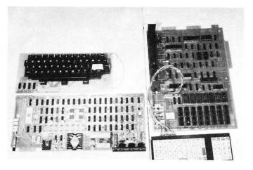
Photo 2. Front-runners: TRS-80 CPU and keyboard, left. PET's CPU and keyboard, right.
