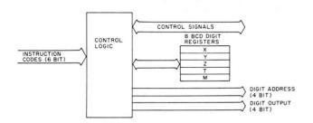
Fig. 2. MM57109 arithmetic processor functional logic.
