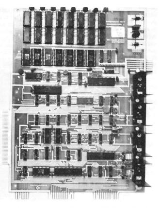
Photo 8. PET's brain: Top 16 chips are RAM. Seven ROM chips below contain operating firmware. Power supply and cassette #1 are along right side. Output ports are along bottom (rear). BUS and memory expansion are at left.
