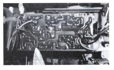
Photo 7. All of the cassette record, playback and erase electronics are on this single small PC card.
