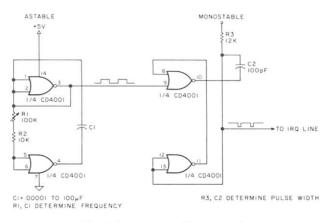
Fig. 1. Interrupt-oscillator circuit.
