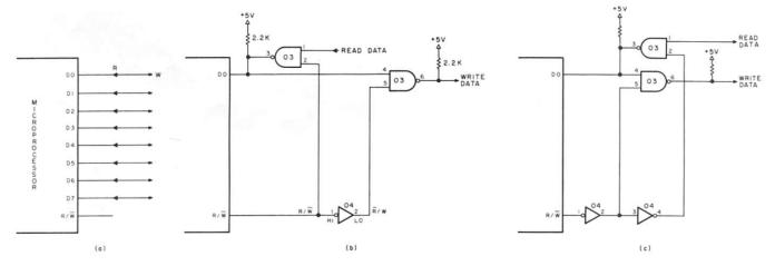
Fig. 7. Traffic control on the data bus.
