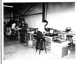
The CRT and CPU units are tested here as they are completed.
