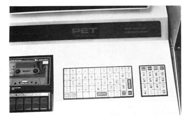
Photo 4. PET's controversial "calculator" keyboard, with quasistandard key placement and conventional calculator number pad. Note variety of graphic symbols available with shift. Lowercase is also implemented (see text).
