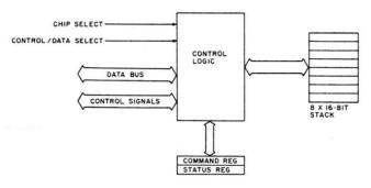
Fig. 7. AM9511 arithmetic processor functional logic.
