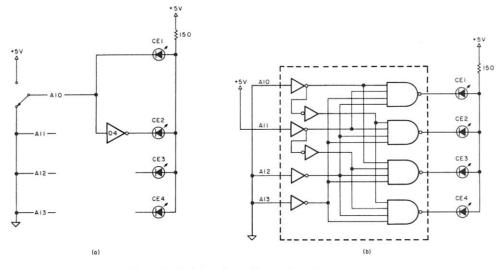
Fig. 4. Delimiting the address decoding problem.
