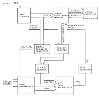
Fig. 1. Block diagram of the A/D converter.
