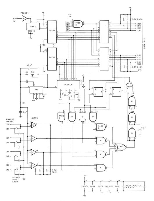
Fig. 2. Schematic of A/D converters.
