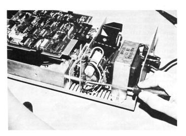
Disk drive assembly. The power supply is assembled to the disk drive assembly with two spacers and screws on each side. The unit is then connected to the case.
