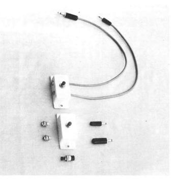
Photo 3. Small case with mounted jacks.
