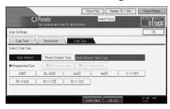
$8^1/_2"\times11"$  indicates LT.  $8^1/_2"\times14"$  indicates LG. 11"×17" indicates DLT.
