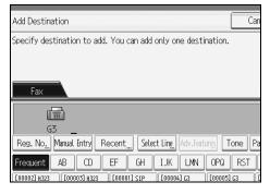
You can switch the transmission type between fax/IP-Fax and Internet Fax by pressing **[Fax]** or **[Internet Fax]**.
