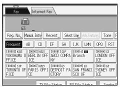
Press **[Fax]** or **[Internet Fax]** to switch the transmission type between fax/IP-Fax and Internet Fax.
