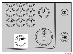
The machine stops scanning.
