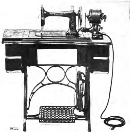
TYPE DSS 1/30 H.P. FORM HC MOTOR—HIGH ARM TYPE
