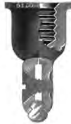
Diagram Showing How The Clamping Ear Holds Grooved Trolley Wire
