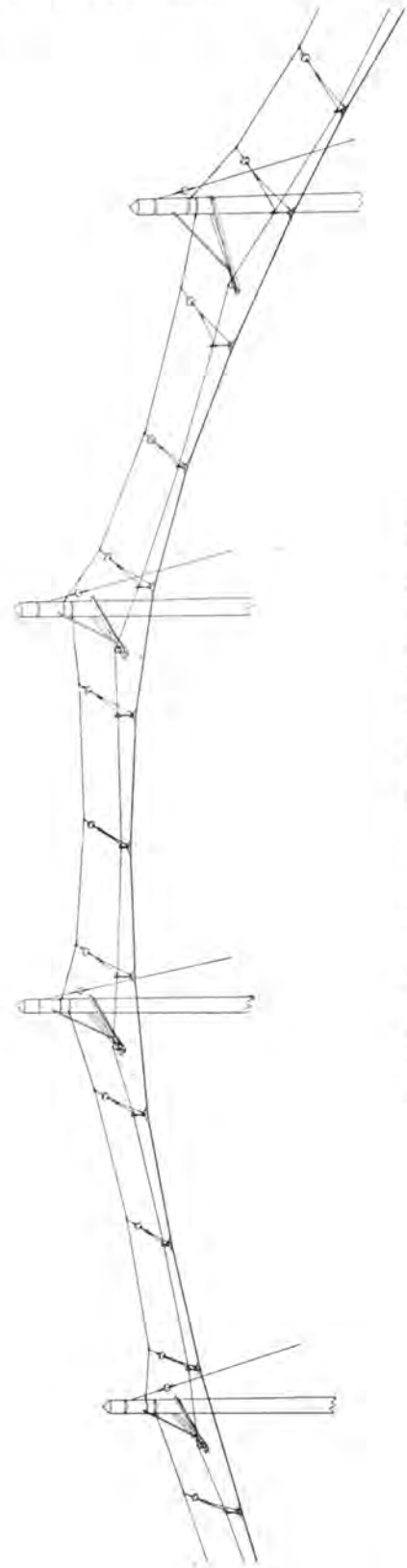
Single Track Curve Construction—With Backbone between Line Poles
