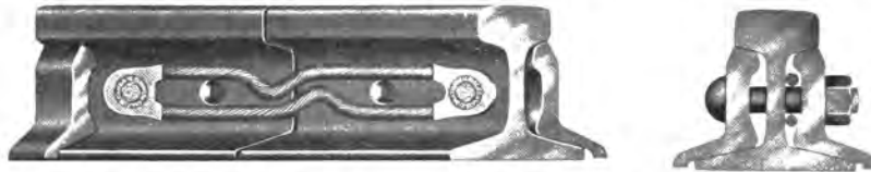
T Rail Bonded with one Form F-5 Bond, Spanning Both Inner Bolts
