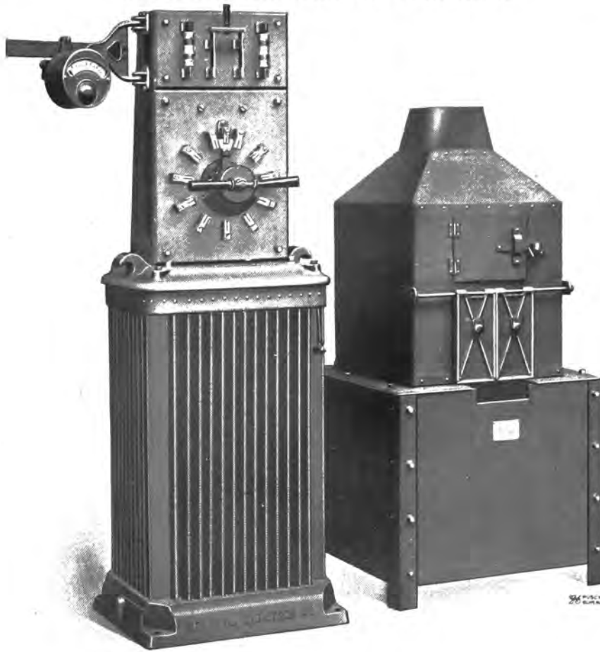
Fig. 1. 25 KW. ELECTRIC HARDENING FURNACE OUTFIT
