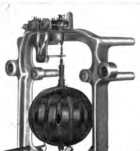
INTERIOR OF THOMSON WATTHOUR METER TYPE C-6 SHOWING SMALL COMMUTATOR AND GRAVITY BRUSHES
