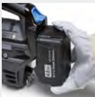
Slot-in battery with release button
