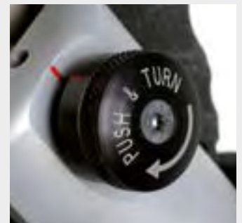
Detail of the quick jaw change device.
