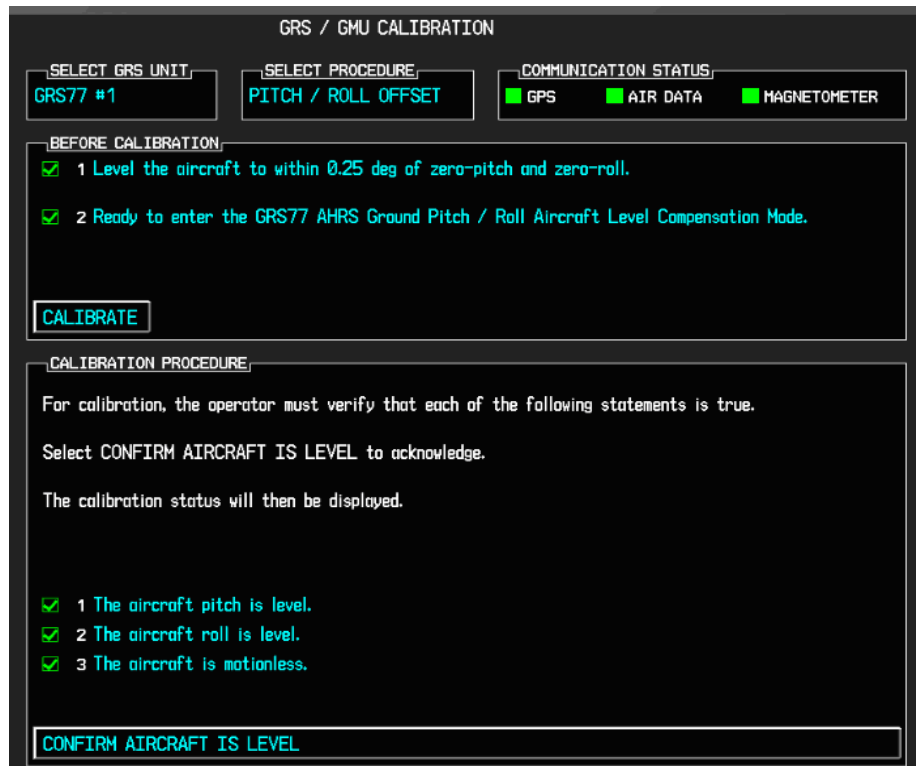
Figure 5-4, GRS/GMU Calibration Procedure
