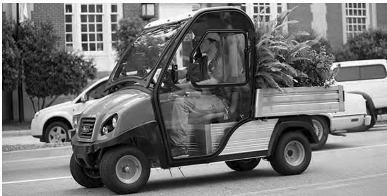
Club Car's Carryall electric, low speed vehicle has a total capacity of 1,250 pounds.
