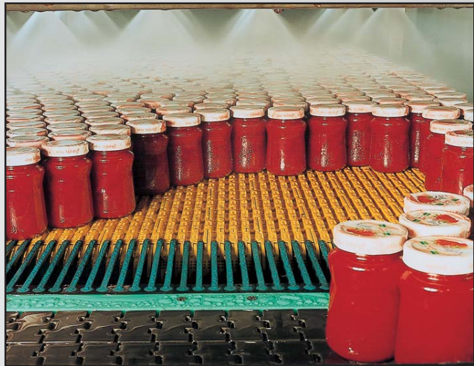
GLASS JARS PASTEURIZING ON 2500 BELT
