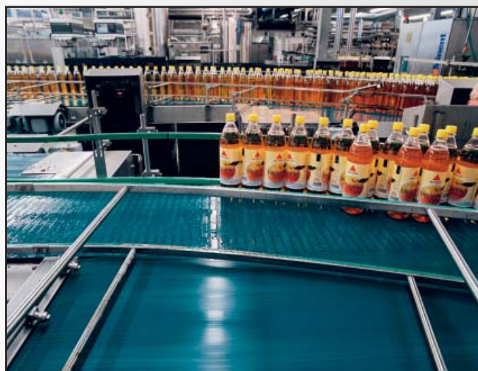
PET BOTTLE CONVEYOR WITH 1000 FLAT TOP BELT
