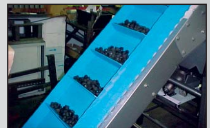
CONFECTIONARY ELEVATING ON 2015 BELT
