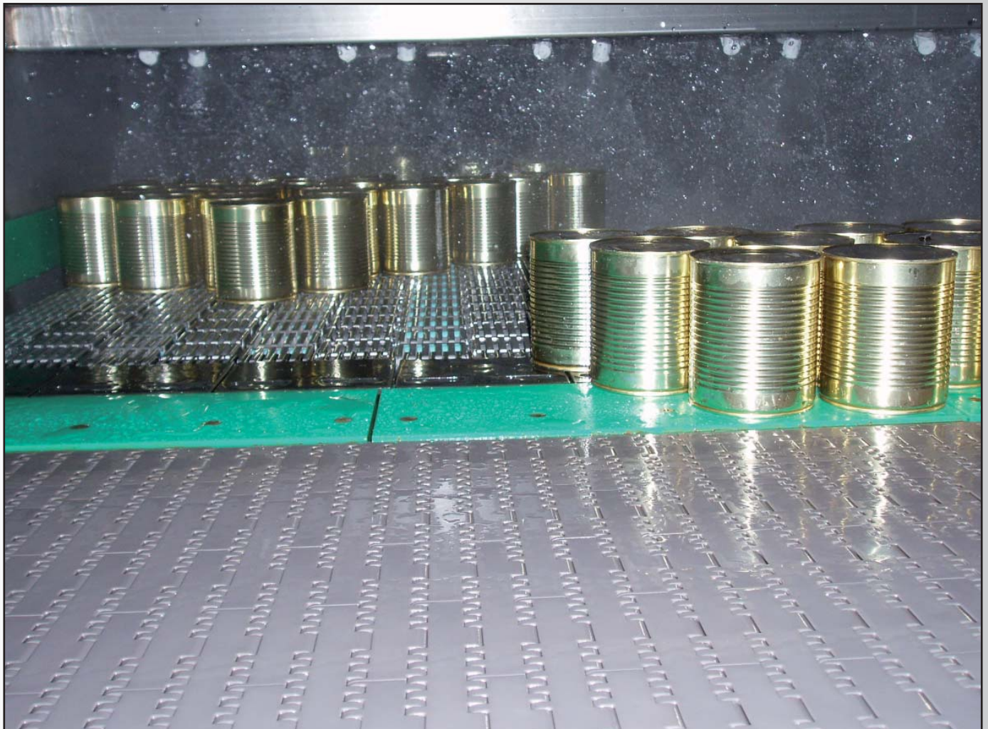
FORTREX 9227 BELT IN A FOOD TUNNEL PASTEURIZER
