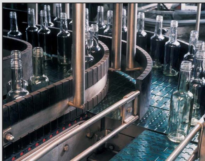
GLASS BOTTLE MANUFACTURING ON 1005 FLAT TOP BELT
