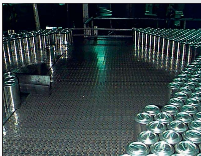
CAN WASHER DISCHARGE WITH 5936 BELT
