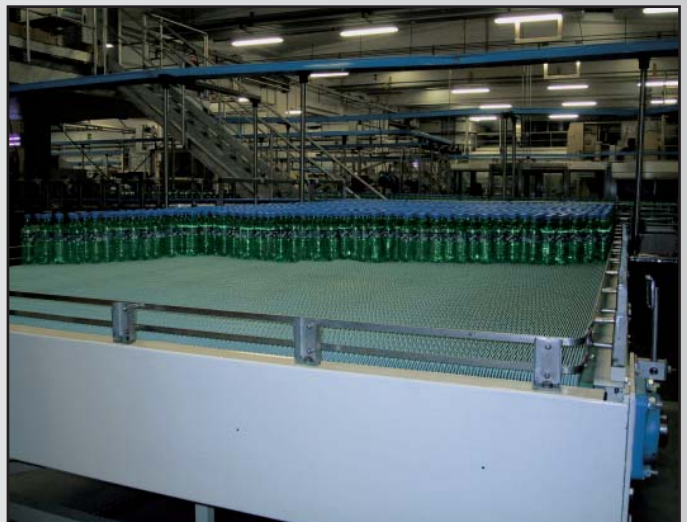
BOTTLE ACCUMULATING ON 2000 BELT
