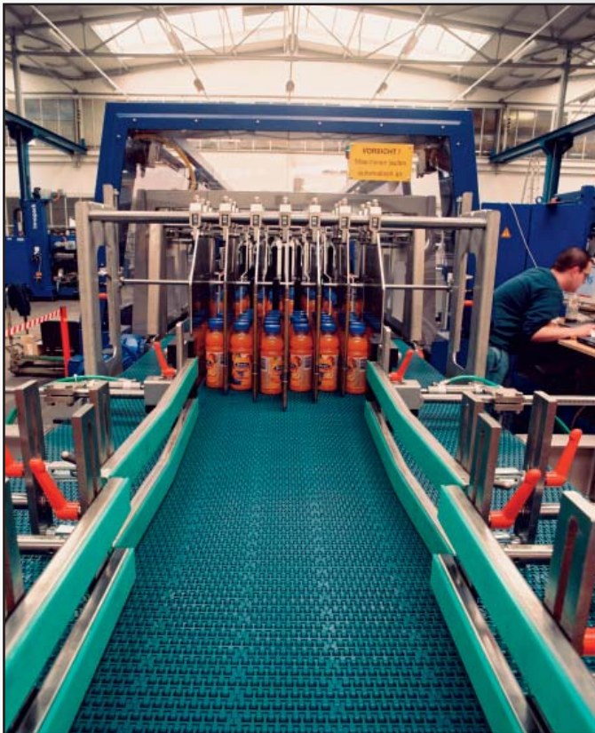
SMALL BOTTLE CONVEYOR WITH 500 BELT
