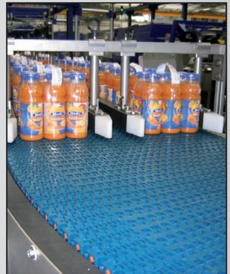
BOXES CONVEYED THROUGH CURVE WITH 1285 BELT
