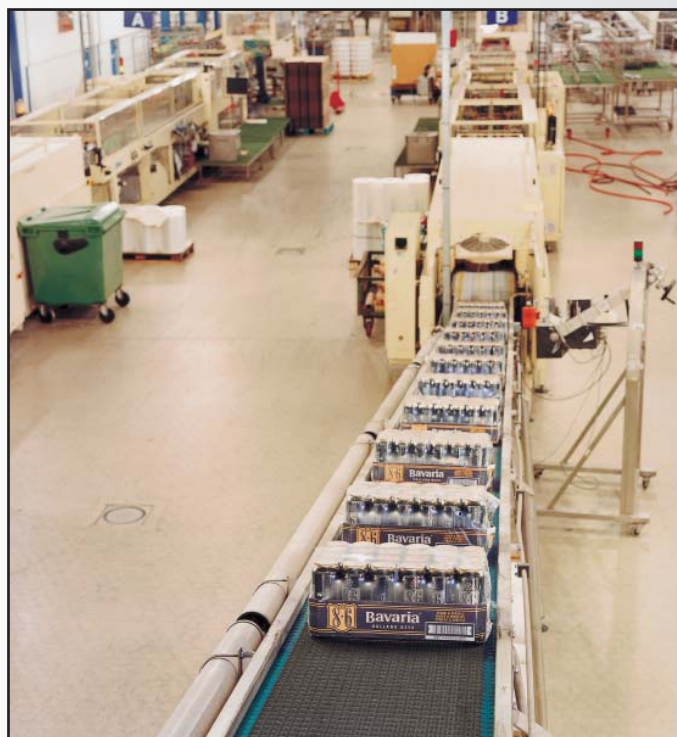
TRAY CONVEYOR WITH 1005 SUPERGRIP BELT
