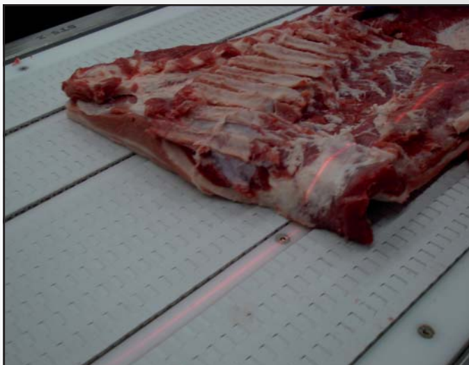
515 BELT ON INFEED OF AUTOMATIC PORK TRIMMER
