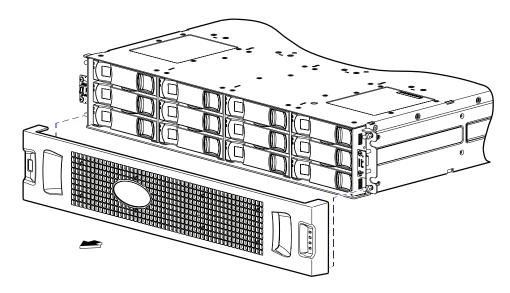
2. While holding the bezel in one hand, gently slip your thumb or index finger between the top of the filter frame and its foam insert on the back side of the bezel.
