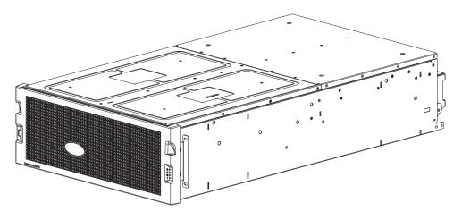
5. Gently push-fit the two ear cover areas of the bezel (interior sleeves) onto the ball studs to secure the bezel in place.
