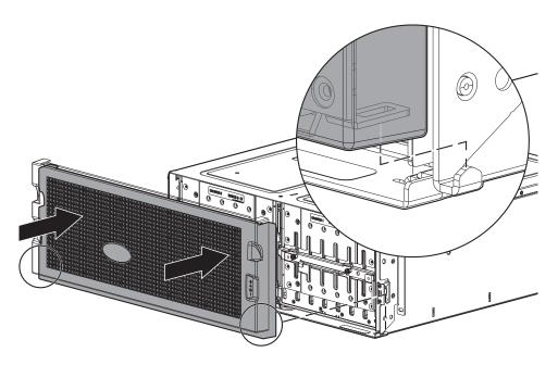
4. Face the front of the chassis, and while supporting the base of the bezel, gently slip the integrated ear covers onto the push-fit ball studs, taking care to guide the LED indicators through bezel openings.
