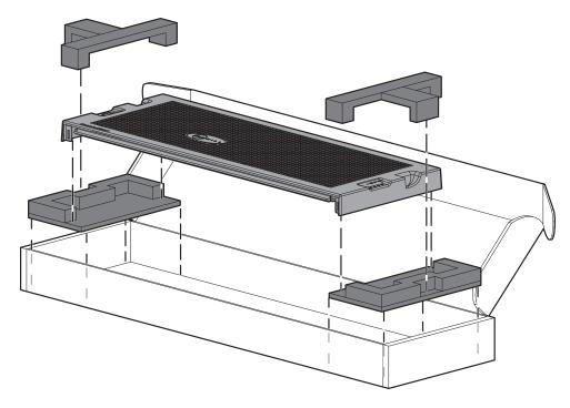
Once you have removed the bezel assembly from its foam-packed box, examine it carefully, to verify that it is properly configured (with or without an air filter) to address your site requirements.
