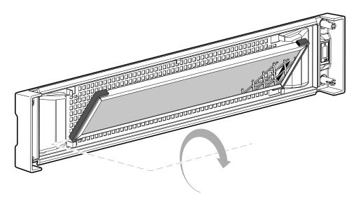
4. Carefully extract the air filter from the bezel.
