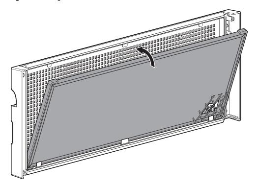
Once properly seated — and revolved into position — the installed air filter should appear as shown in the figure below; albeit with visible foam-retaining mesh in front of the shaded foam insert (the mesh is only partially shown in the illustrations provided in this document).
