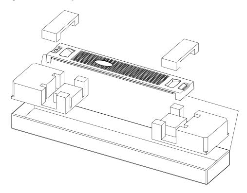
Once you have removed the bezel assembly from its foam-packed box, examine it carefully, to verify that it is properly configured (with or without an air filter) to address your site requirements.
