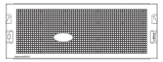
Figure 15: Optional air filter sub-assembly - front view
