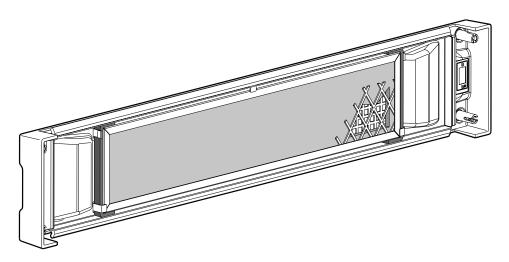
**Note:** Once the air filter is successfully installed within the bezel, you can reattach the bezel to the front face of the chassis.
