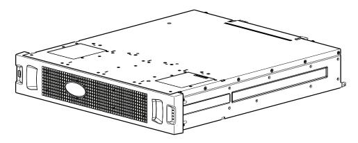
5. Gently push-fit the two ear cover areas of the bezel onto the ball studs to secure the bezel in place.
