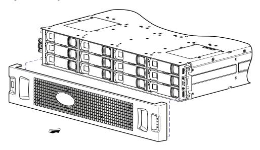
4. Face the front of the chassis, and while supporting the base of the bezel, gently slip the integrated ear covers onto the push-fit ball studs, taking care to guide the LED indicators through bezel openings.
