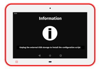
When the USB storage device is unplugged this message is displayed for less than 5 seconds.
