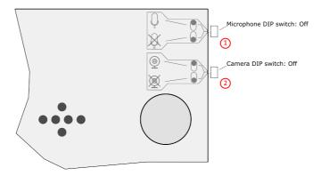
Example of configuration when the microphone 3 and the camera 4 peripherals are activated:
