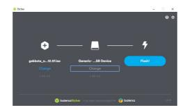
Press on the Flash! button and wait that the micro SD card burning has completed.
