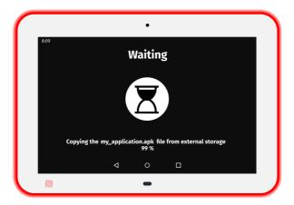
Unplug the USB storage device. This message should be displayed for few seconds, the time for the AQS to install the APK.
