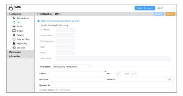
To use an automatic proxy server configuration, select the Automatic proxy configuration in the Proxy server drop down list then enter the PAC file URL allowing to get automaticall the proxy server configuration.
