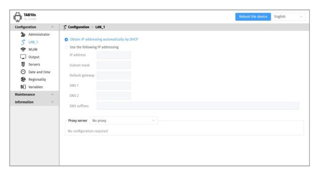
The connection to the Web configuration user interface with the device IPV6 address, computed from the device MAC address value, is supported. For example, if the LAN\_1 MAC address of the device is 00-1c-e6-02-27-bf, type the URL http://[fe80::21c:e6ff:fe02:27bf]/ or type http://[fc00::21c:e6ff:fe02:27bf]/ in a Web browser. The routable prefix is depending on your network configuration.
