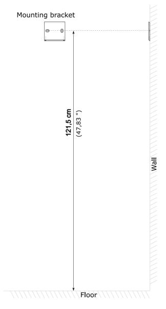
△ The TAB10s device is designed to be installed in landscape mode only.
