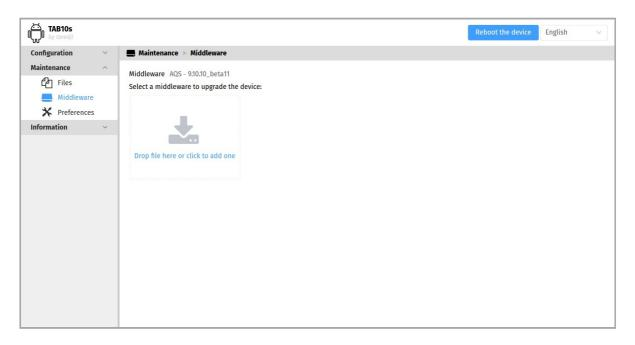
Drop your .fqs file in the Drop file here or click to add one location or click on the button Drop file here or click to add one to pick up the appropriate firmware, then click on the send button to update the AQS (for AOSP Qeedji System) version of your device. Wait a few minutes, the time to install the new middleware version. Go back to the Administration console user interface and check that the AQS version number of the device has changed.
