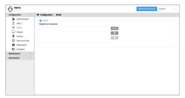
Select one of the detected WIFI spots SSID and press on the Add button.
