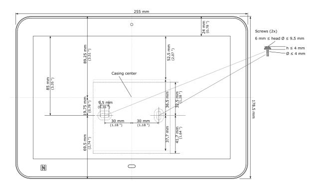
This mounting bracket can be fixed using screws (recommended for walls with pierceable material).
