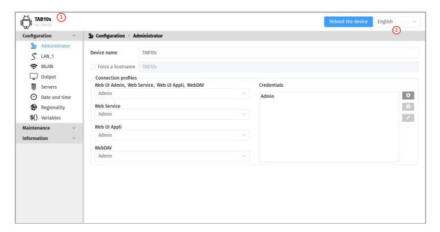
After you have changed and saved all your settings in the different panes, be sure to perform a device restart by clicking on the Reboot the device 2 button so that your changes are fully reflected.
