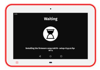
After the AQS firmware installation, the device is rebooting automatically once. This message is displayed while the device has not yet restarted.
