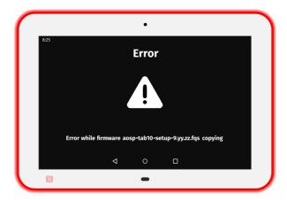
One of these messages could occur when the AQS file is corrupted or when the USB storage device has been removed when the copy was still in progress. If required, download again the AQS version (.fqs) from the Qeedji Website and try again. If the problem persists, contact <a href="mailto:support@qeedji.tech">support@qeedji.tech</a>.
