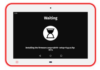
After the AQS version installation, the device is rebooting automatically once. This message is displayed while the device has not yet restarted.
