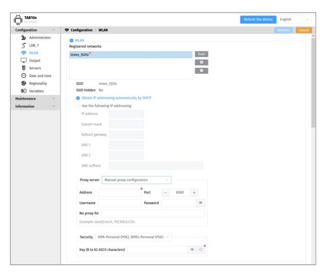
To use an automatic Proxy server configuration, select the Automatic proxy configuration in the Proxy server drop down list then enter the PAC file URL allowing to get automatically the proxy server configuration.
