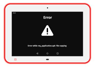
This error message is displayed for ten seconds when the APK is corrupted or when the USB storage device has been removed when the copy was still in progress. Try again. If the problem persists, you can contact <a href="mailto:support@qeedji.tech">support@qeedji.tech</a>.
