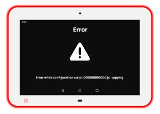
This error message is displayed for ten seconds when the configuration script contains a Javascript syntax error. Double check that the configuration script content is consistent for the TAB10s device.
