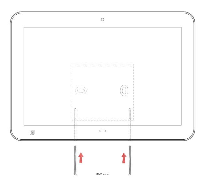
⚠ When installed on the NAPOE109kt or NAPOE109ft products having a mounting bracket with a POGO connector, before mounting the screws to lock the device, check that the TAB10s device is installed on the NAPOE109kt or NAPOE109ft products stricly on the vertical position else some unexpected power supply issue could be faced.
