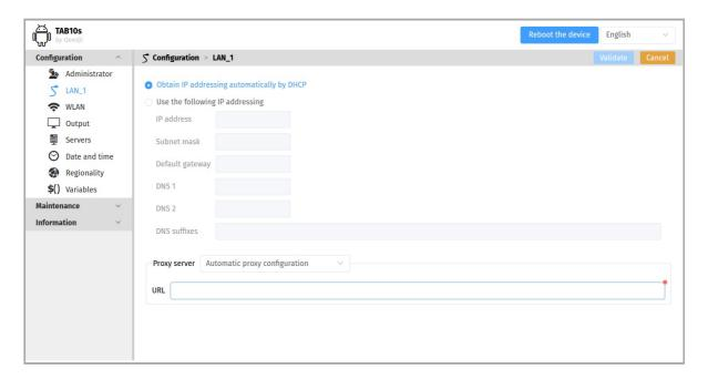
The Automatic proxy configuration is not supported on the LAN\_1 interface.
