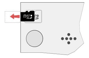
r It may be required to lift the micro SD card so that it can enter into the connector. Press a little on it to tilt it.
