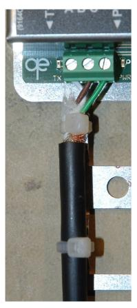
The simplest way to accomplish this is to remove the outer insulation of the cable and to fold down the screen on the outside of the insulation and to secure the cable with the straps supplied.
