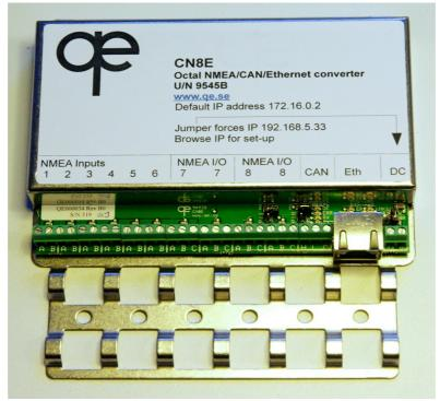
Note! The default ip address of the unit is 172.16.0.2 from SW 99061.0.1.18 onwards!
