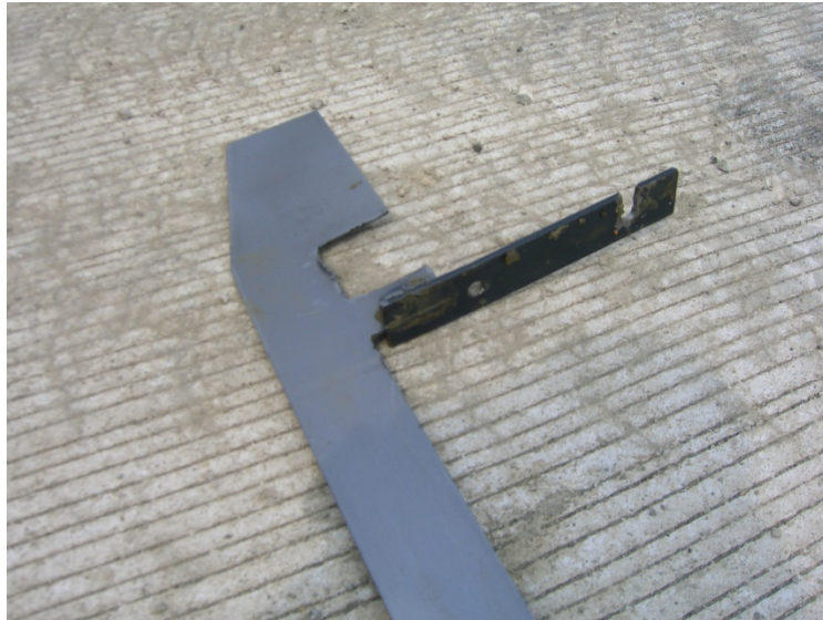
The removable joint-forming knife used for creating longitudinal joints
