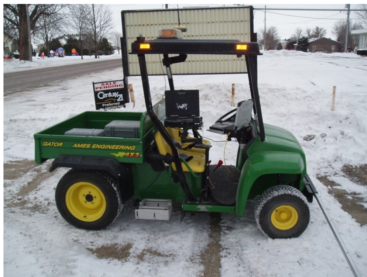
Figure 33. GPS receiver and laser profiler located on the top of the John Deere Gator
