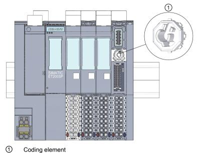
Figure 8-2 Changing the type of an I/O module
