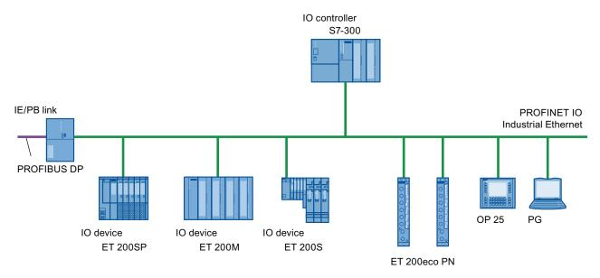
Figure 2-1 Typical configuration of PROFINET IO
