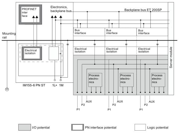
Figure 5-2 Potential relationships for ET 200SP with IM 155-6 PN ST
