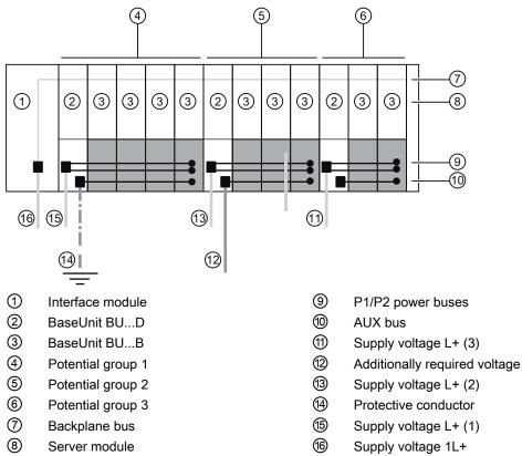
Figure 3-3 Placing the BaseUnits
