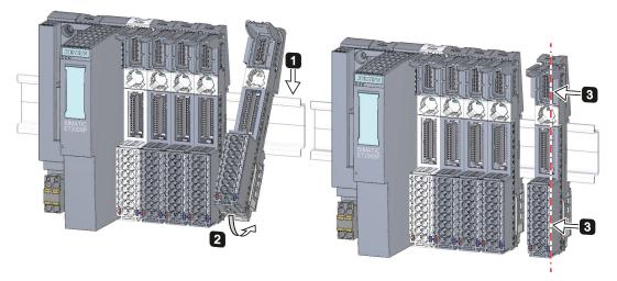
Figure 4-3 Installing a BaseUnit
