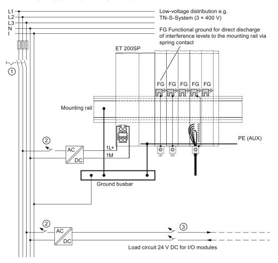
Figure 5-1 Operating the ET 200SP with grounded reference potential
