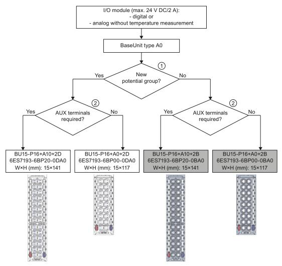
① Light BaseUnit: Configuration of a new potential group, electrical isolation from adjacent module on the left. The first BaseUnit of the ET 200SP is always a light BaseUnit for feeding the supply voltage L+.
