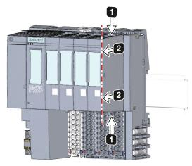
Figure 8-1 Pulling I/O modules
