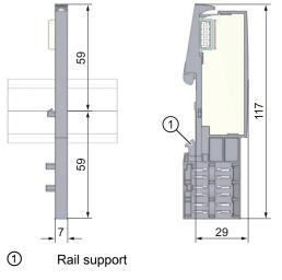
Figure A-1 Server module dimensional diagram
