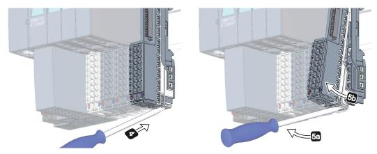
Figure 8-3 Replacing the terminal box on the BaseUnit
