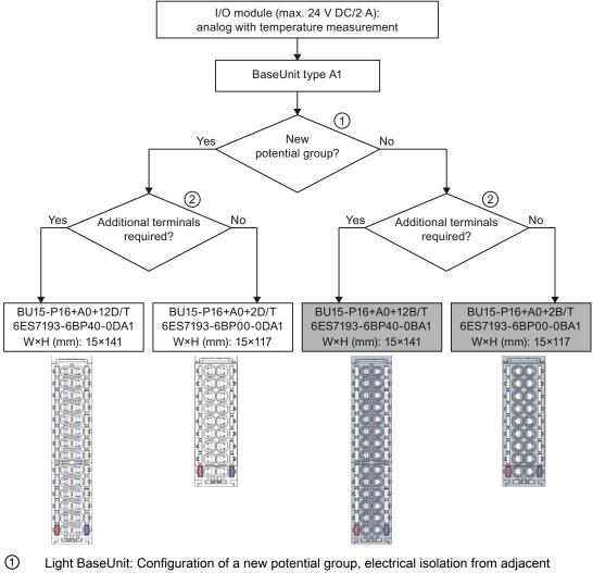
(1) Light BaseUnit: Configuration of a new potential group, electrical isolation from adjacent module on the left. The first BaseUnit of the ET 200SP is always a light BaseUnit for feeding the supply voltage L+.
