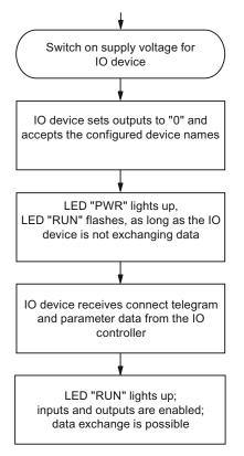
Figure 7-1 Startup of the ET 200SP on PROFINET IO
