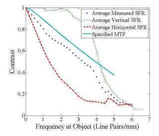
**Fig. 1** Modulation transfer function of the imaging system with the object at a 2.2-cm range.
