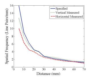
Fig. 2 Maximum resolvable spatial frequency (at the object plane) versus object distance.
