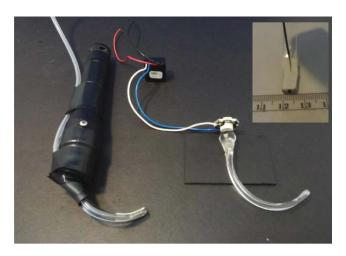
**Fig. 5** The full prototype is shown on the left and the LED, lens, and light guide assembly is shown on the right, with the tip shown with a ruler for scale (inset).
