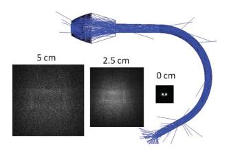
**Fig. 4** Optical simulation of light pipe efficiency showing light distribution for several distances from the tip.
