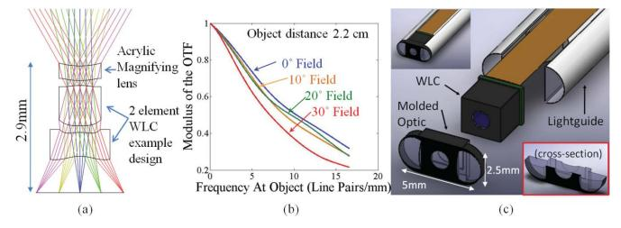
Fig. 9 (a) Raytrace diagram and (b) MTF for the modified WLC imager. (c) Shows the conceptual drawing of the entire laryngoscope tip, including the WLC, light pipe, and molded optic.
