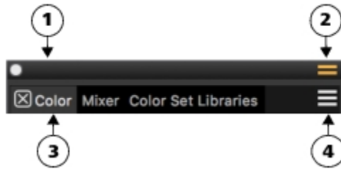
A typical palette features a header bar (1), a Palette Drawer button that lets you turn a palette drawer (2), panel tabs (3), and a Panel options button that allows you to access a series of related commands (4).
