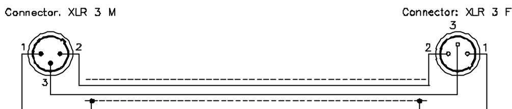
figure 2 LF cable for coupling two amplifiers DPA 41xx
