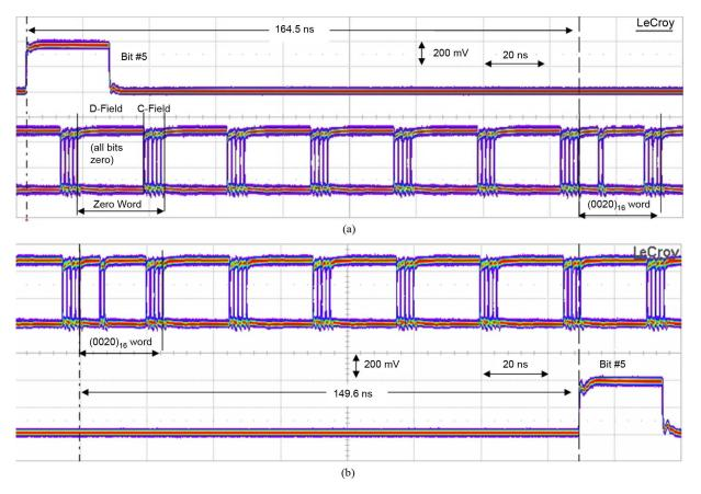
Fig. 11. Oscilloscope screen-shots showing the latencies of the transmitter and of the receiver. (a) Upper trace: transmitted payload bit. Lower Trace: CIMT encoded serial stream. (b) Upper trace: CIMT encoded serial stream. Lower Trace: received payload bit.
