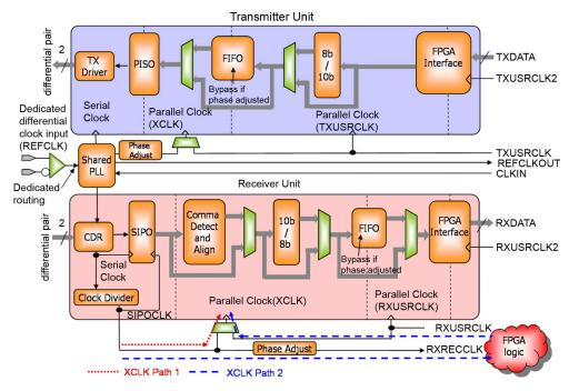
Fig. 4. Simplified block diagram of Xilinx GTP transceivers. Half a tile is shown.
