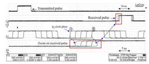
Fig. 3. Latency between transmitted and received pulse for different clock skews.
