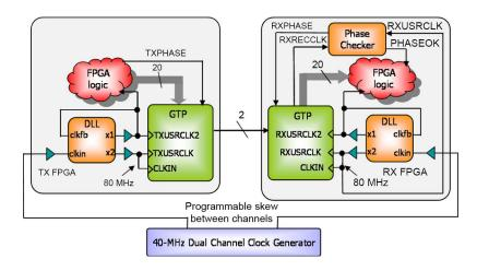
Fig. 7. Adopted clocking scheme for the GTP transmitter and receiver for synchronous operation.
