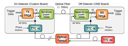
Fig. 1. Simplified block diagram of the serial link setup in L1 ATLAS barrel muon trigger.
