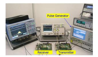
Fig. 9. Experimental setup for latency tests.
