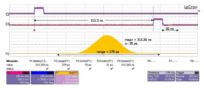
Fig. 10. Histogram of the latency of the link. Topmost trace: transmitted payload bit. Second trace: corresponding received bit. Down: histogram of the latency.
