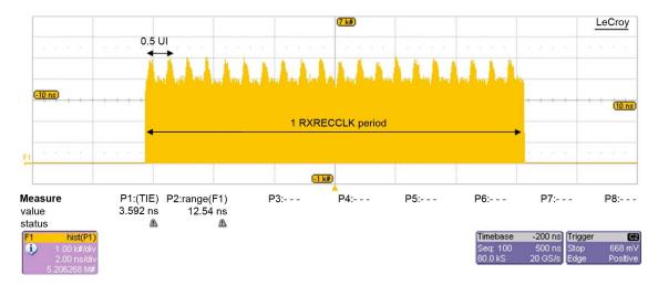
Fig. 8. Histogram showing the relative phase between RXRECCLK and the reference clock when  $\Delta \phi$  does not satisfy the requirements of the phase align circuit.
