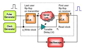
Fig. 2. Synchronous serial link with skew on clock distribution.
