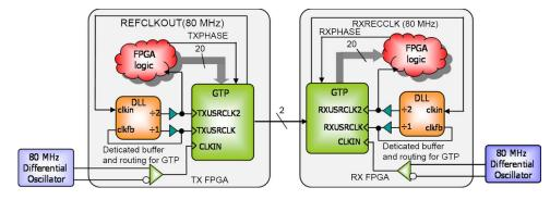
Fig. 5. Recommended GTP clocking scheme when using phase alignment circuits.
