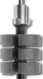
The XXX Slotted armature was designed to exploit the increased magnetic field of the D3's new 6.0v wet magnets and innovative can design. This combination of XXX armature and D3 setup makes for a more efficient motor without sacrificing top end. The D3 produces the same torque as the older D2 motors but with an increase of usable rpm. The power band has also been widened to make the D3 more drivable over a wide variety of track and car conditions.
