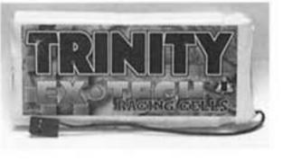
you are now operating your radio on 9.6 volts. This low voltage can sometimes contribute to power, range and frequency problems. To help eliminate this problem we have developed a 9 cell rechargeable pack for both of these popular radios. These packs increase the voltage to 10.8 volts which is a lot closer to the 12 volts the radio was designed to operate on.
