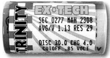
Trinity VIS EX-TRA cells come from the same cell pool from which we make up our World-Tech battery packs, so only the finest cells available in R/C are used. These cells have already been through 20, 25 and 30 amp cycling stages to insure that their discharge curves and output will be suitable to the type of racing they will eventually see in your R/C car.
