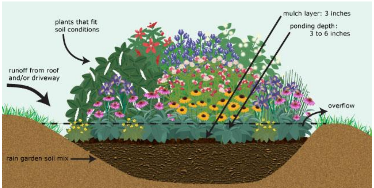
Figure 5-4. Typical Rain Garden Design
