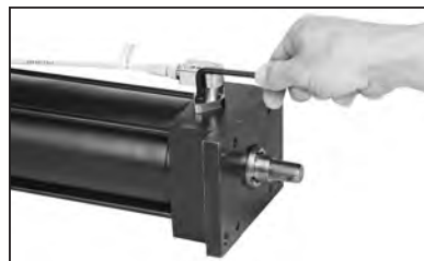
Bolt sensor to cylinder.
