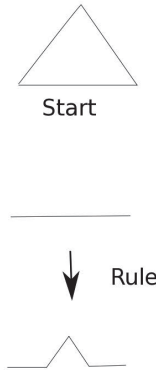
Fig. 2.42 Start string F - -F - -F and L-rule F \rightarrow F + F - -F + F with \delta = 60^\circ
