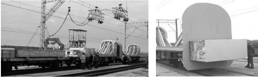
Fig. 7. Experimental test: Physical set-up and honeycomb structure
