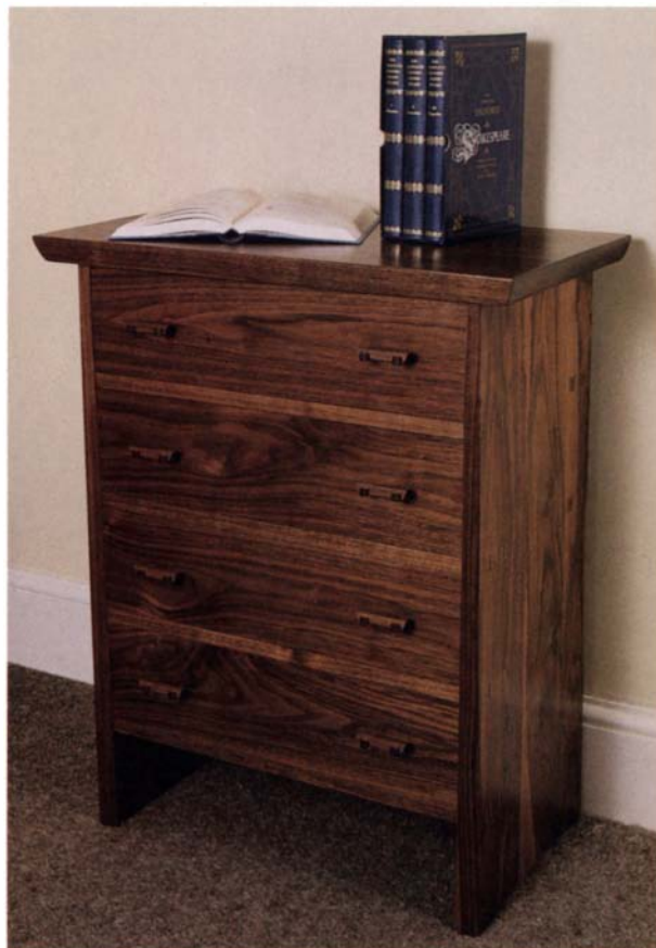
Subtle geometry in this chest of drawers built by Malcolm Vaughan accentuates both the wood and the form, reflecting the honesty in materials and manufacture that is the hallmark of the Arts-and-Crafts style. Vaughan boldly pierced the bureau's side with the through-tenon ends of the drawer dividers, contrasting black walnut tenons with pear wedges.
