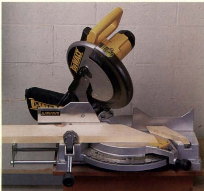
The carriage on DeWalt's DW705 doesn't slide, but its 12-in. blade does handle a full range of miter and compound angle cuts in stock up to 5½ in. wide.
