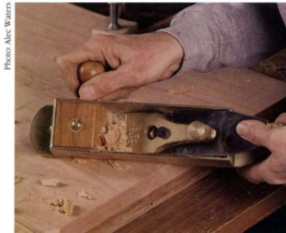
Equally adept at shaving end grain, edge jointing or smoothing burls or bird's-eye maple, the Lie-Nielsen #9 is a versatile heavyweight. Because its sides are square to the bottom, the #9 is also the ideal plane to use with a shooting board for trimming miters.
