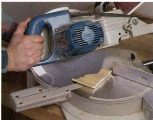
Cutting compound angles on crown molding is a straightforward process on a sliding compound miter saw like the Makita LS1011 shown here. Rotate and lock the turntable base for the miter angle, and then tilt and lock the head at the desired bevel angle.
