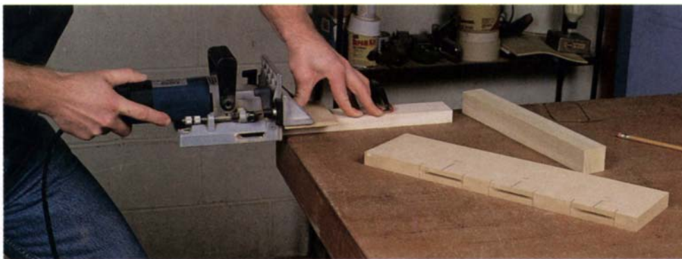
Cutting an offset joint using a shim spacer, the author kerfs a table apron that will be set back from the face of its leg by the thickness of the shim. The template in the foreground helps to lay out the kerf in the apron's narrow end.
