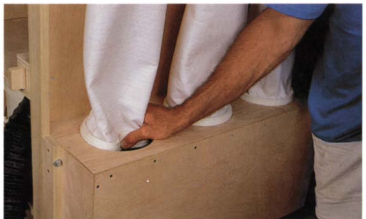
Tube filters snap easily into place, and the felt seal's groove fits snugly over the 1/4-in.-thick plywood dustbin lid. Because the bag's open end hangs down, excess filter cake that accumulates on the inside of the bag simply falls into the bin below.
