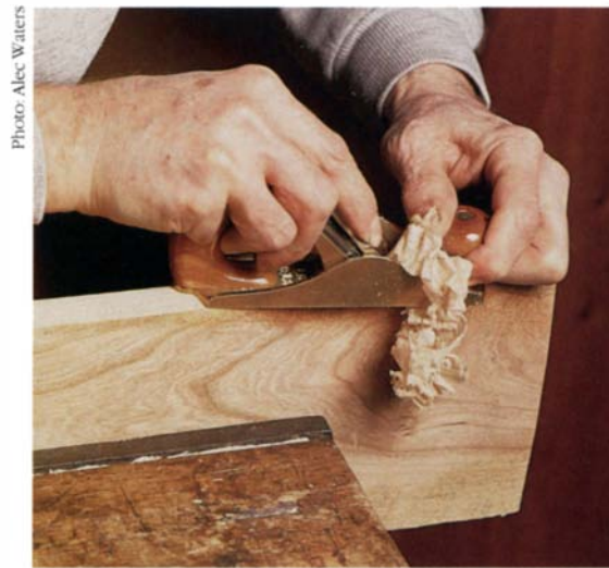
A two-handed grip is required by the bench-plane configuration of the Lie-Nielsen #1 even though it is the size of a block plane. Maurice Fraser demonstrates use of the tool on the edge of a board.
