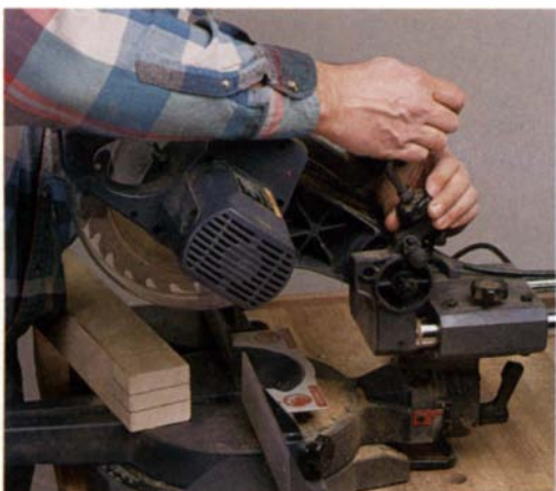
Ryobi's forward-positioned tilting mechanism is convenient, and its large printed scale and fine cursor make it easier to set precise bevel angles.
