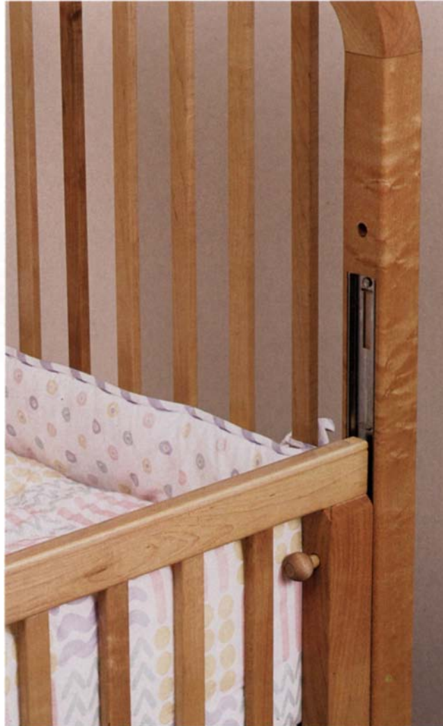
To drop the side, the author adapted standard drawer slides. A pair of spring-loaded pins, one on each end of the crib, latch the side in its up position.
