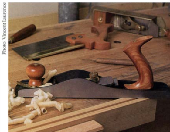
Low-slung, precisely machined and outfitted with a hefty razor-sharp blade, Lie-Nielsen's new low-angle jack is a tremendously versatile plane. Whether on pine, oak or maple, edge, face or end grain, this plane left a glass-smooth finish.
