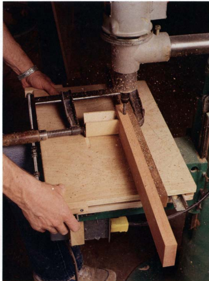
Ideal for mortising, this shopmade sliding table advances a mahogany stile under a fluted stagger-tooth bit chucked in an overarm router. Author Mac Campbell secures the workpiece to the fence with a block of scrap and a C-clamp.
