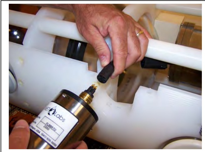
Figure 6.2-5: Connecting the Sensor Cable
