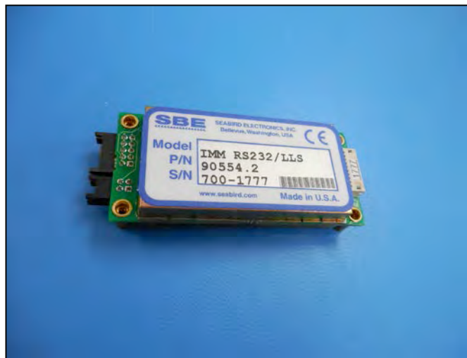
Figure 11.1-1: Sea-Bird IMM Modem
