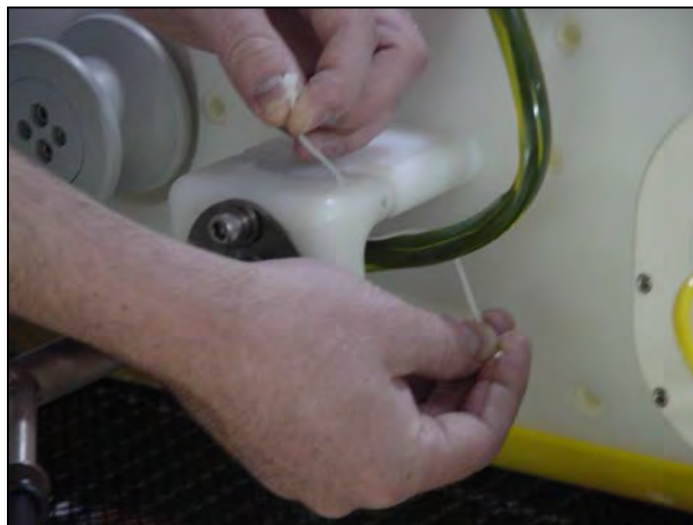
Figure 4-17: Secure Excess Cable
