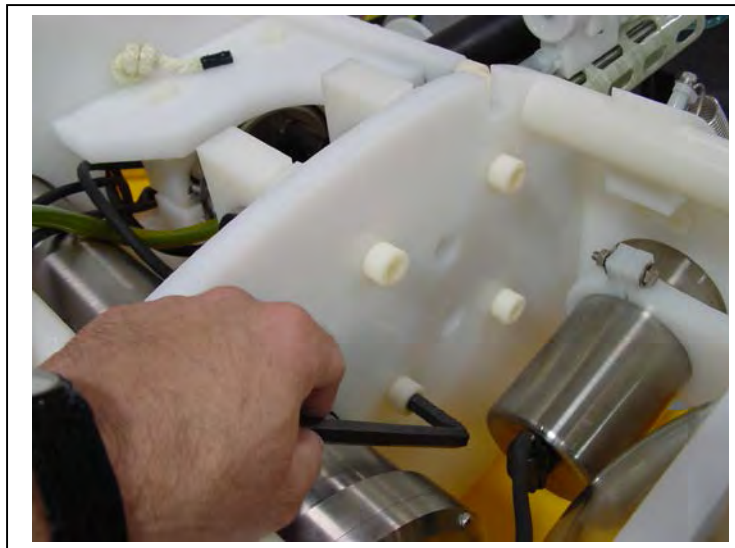
Figure 1.1-10: Loosening the Mounting Plate Screw
