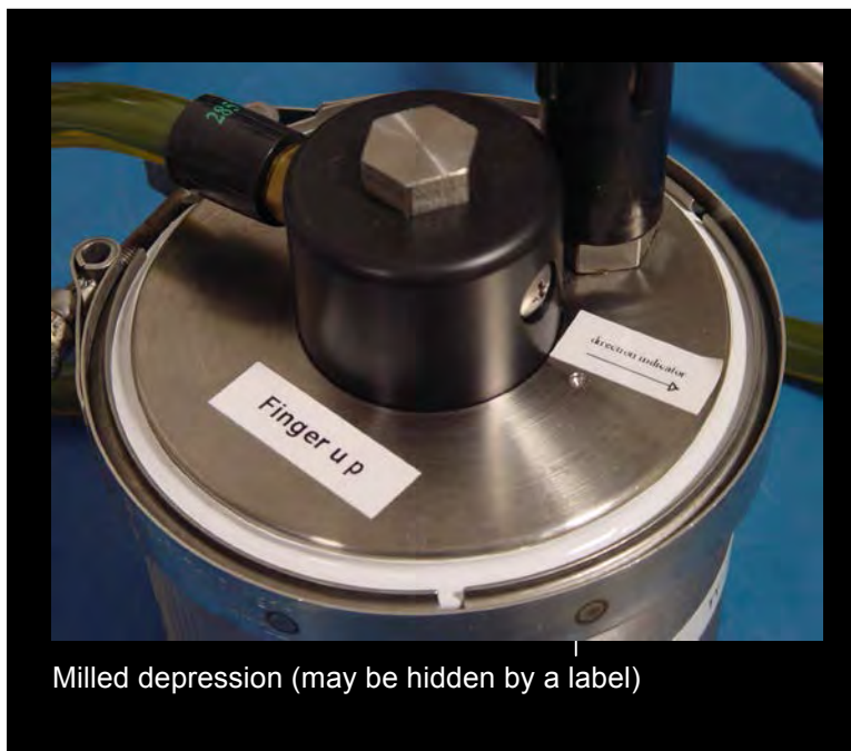
Figure 4-19: Correct Positioning of ACM+ Electronics Housing
