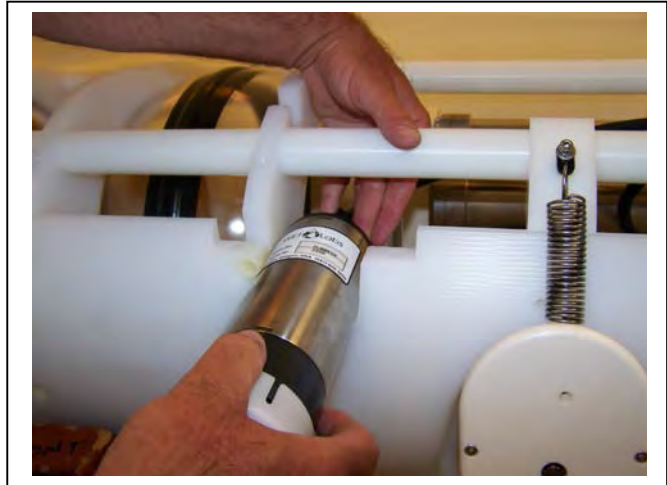
Figure 6.2-6: Placing the Sensor in the Mount
