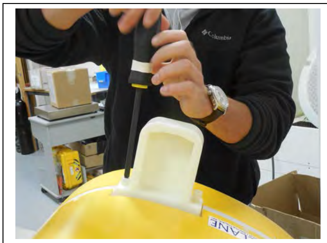
Figure 6.3-11: Tightening Nylon Screws
