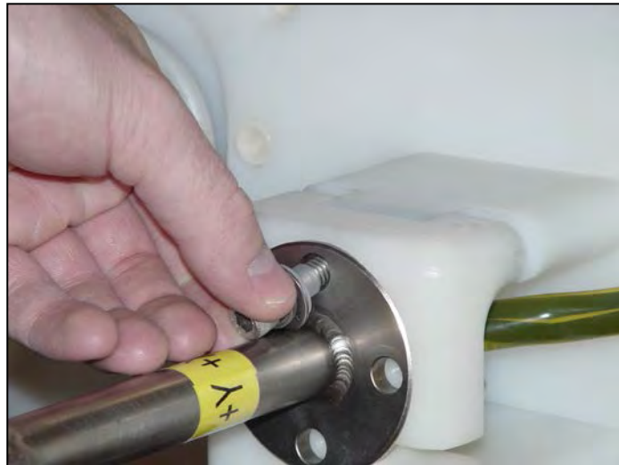
Figure 4-16: Tighten ACM+ Sting
