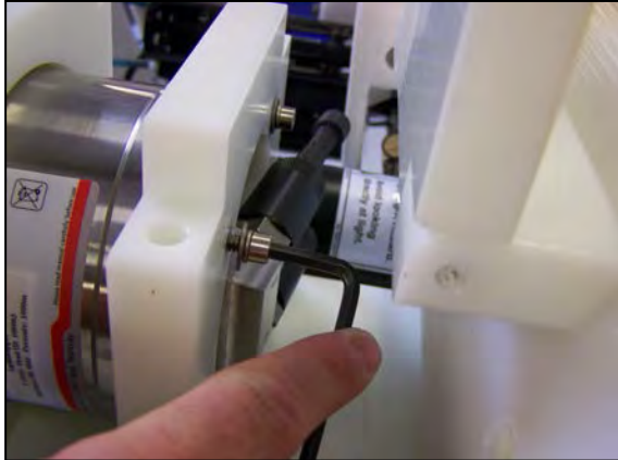
Figure 3.1-22: Loosen Back Screws
