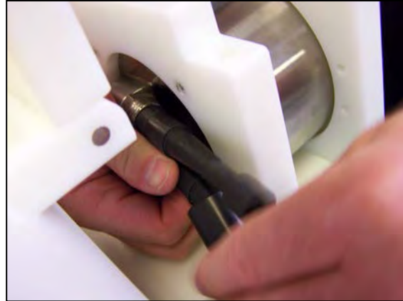
Figure 3.1-23: Detach Bulkhead Connector
