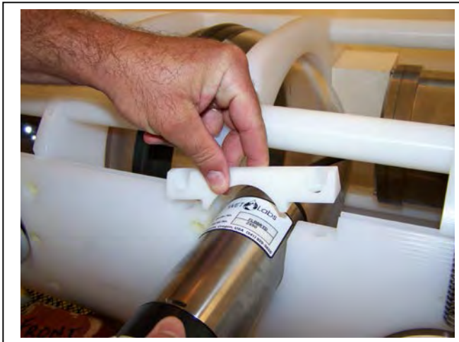
Figure 6.2-7: Placing the Mounting Support
