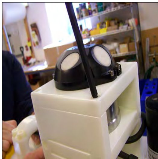
Figure 3.1.28: Tighten Hinge Plate Screws
