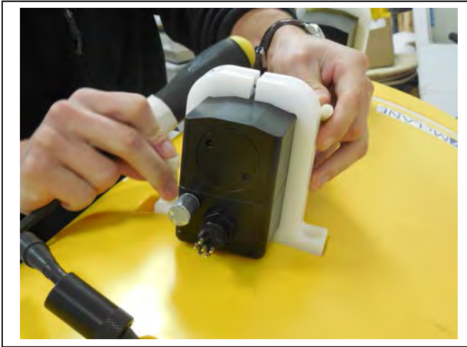
Figure 6.3-13: Securing Top Clamp
