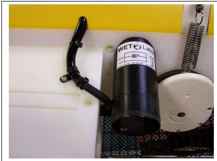
Figure 6-11: BBFL2 Model- Installed
