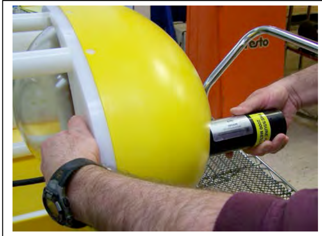
Figure 9-17: Pulling Out Sensor Clamp
