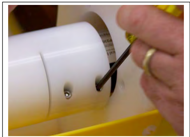
Figure 9-16: Loosening the Clamp Screws
