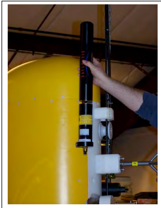
Figure 8-16: Sliding the SUNA into the Sensor Brackets
