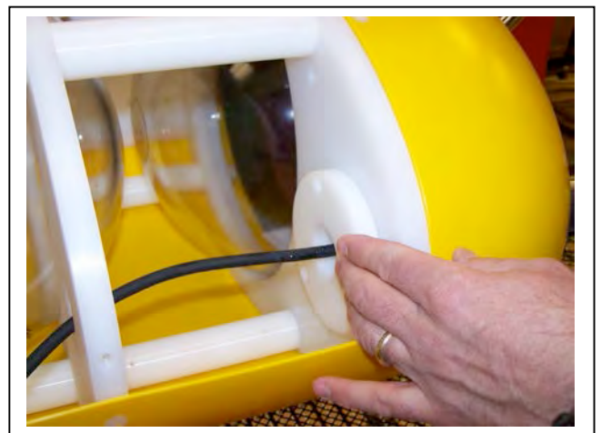
Figure 9-10: Re-inserting the Clamp
