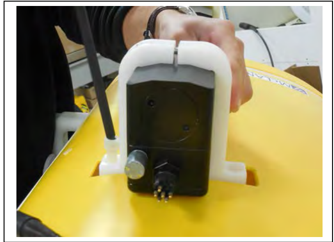
Figure 6.3-14: Tighten Top Clamp Nylon Screws
