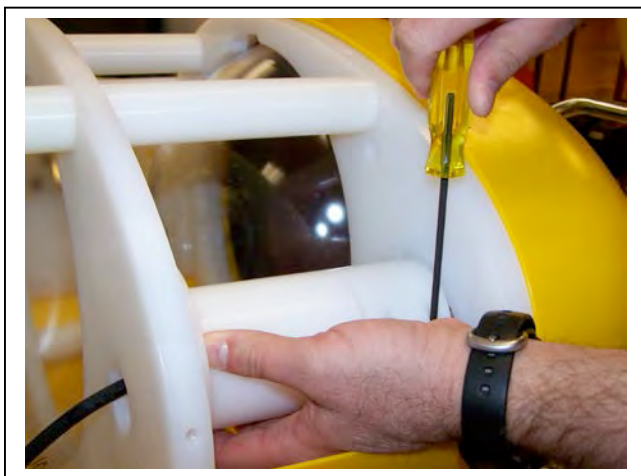
Figure 9-9: Securing the Sensor Clamp
