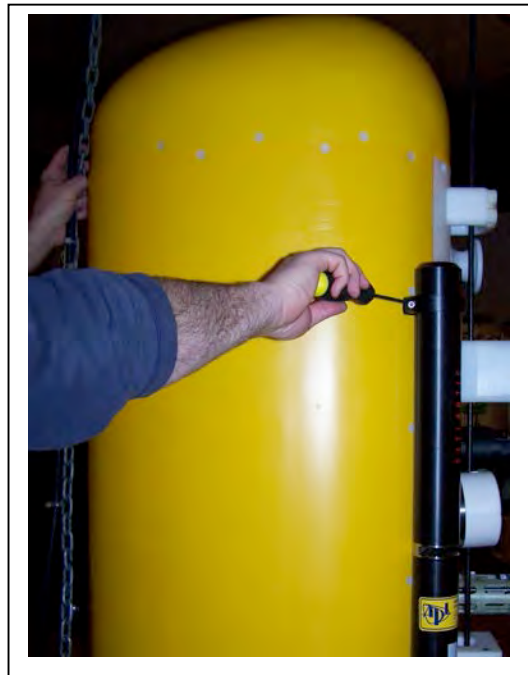
Figure 8-17 and Figure 8-18: Tightening Bottom and Top Mounting Screws
