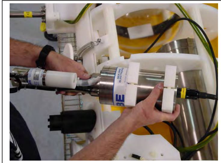
Figure 1.1-11: Lifting the CTD from the Sensor Mount
