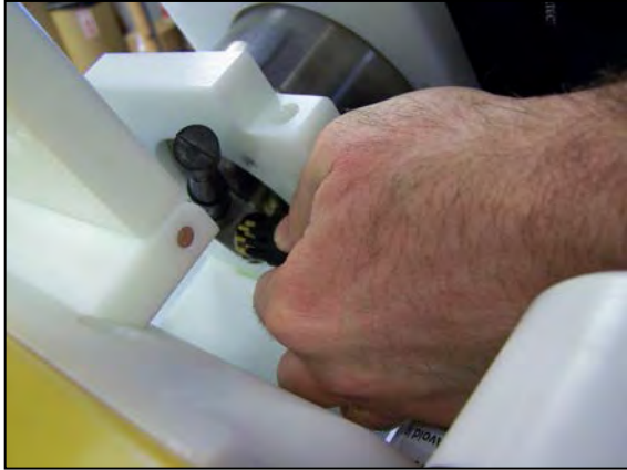
Figure 3.1-24: Reconnect Bulkhead Connector
