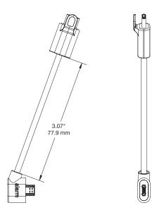
One55/One65/One60 Tablet USB Micro Power Connector (DBT500):
