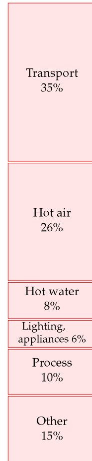
Figure 18.2. Energy consumption, broken down by end use, according to the Department for Trade and Industry.
