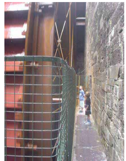
Figure 8.4. A 60 kW waterwheel.
