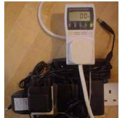
Figure 11.2. These five chargers – three for mobile phones, one for a pocket PC, and one for a laptop – registered less than one watt on my power meter.
