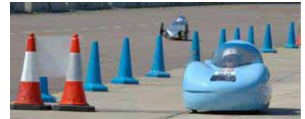
Figure 20.2. Team Crocodile's eco-car uses 1.3 kWh per 100 km. Photo kindly provided by Team Crocodile. www.teamcrocodile.com
