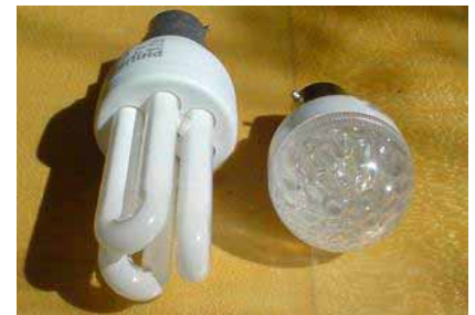
Figure 9.4. Philips 11 W alongside Omicron 1.3 W LED bulb.
