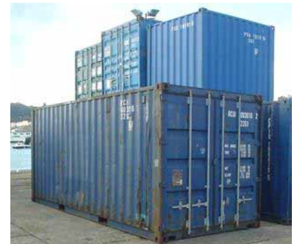
Figure I.4. A twenty-foot container (1 TEU).
