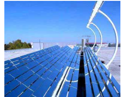
Figure 6.19. A combined-heat-and-power photovoltaic unit from Heliodynamics. A reflector area of 32 \text{ m}^2 (a bit larger than the side of a double-decker bus) delivers up to 10 kW of heat and 1.5 kW of electrical power. In a sun-belt country, one of these one-ton devices could deliver about 60 kWh/d of heat and 9 kWh/d of electricity. These powers correspond to average fluxes of 80 \text{ W/m}^2 of heat and 12 \text{ W/m}^2 of electricity (that's per square metre of device surface); these fluxes are similar to the fluxes delivered by standard solar heating panels and solar photovoltaic panels, but Heliodynamics's concentrating design delivers power at a lower cost, because most of the material is simple flat glass. For comparison, the total power consumption of the average European person is 125 kWh/d.
