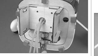
□ 3. Attach a 6" to 7" [152 to 178mm] piece of fuel tubing onto each line coming from the tank. Insert the tank into the fuselage with the correct side facing up as far forward as it will fit.
