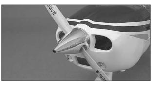
□ 3. Tighten the spinner cone to the backplate using the 4 x 45mm SHCS.
