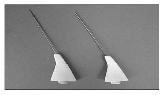
□ 2. Roughen 1/4" [6mm] from one end of each metal antenna wire and clean the area with alcohol. Glue the antennas into the antenna bases as shown. We used thick CA. However, epoxy could also be used.
