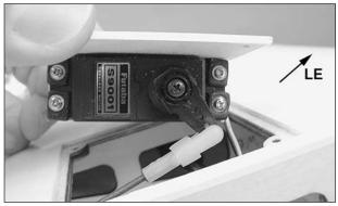
□ □ 3. Slide the pushrod through the access hole in the wing and connect the bent end of the pushrod to the outer hole in the flap control horn using a nylon FasLink. Connect the clevis to the outer hole in the flap servo arm. Put the flap servo hatch cover in place onto the wing. While holding the hatch cover down, use your radio system to test the operation of the flap. Make any adjustments necessary to the position of the clevis on the pushrod or the servo arm.
