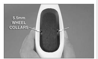
$\Box$  7. Loosely thread a 3 x 4mm machine screw with threadlocking compound into each 5.5mm wheel collar. Reinstall the wheel collars and nose wheel onto the nose gear wire along with the wheel pant. Tighten the screws in the wheel collars onto the flat spots you made on the axle. Confirm that the wheel spins freely on the axle. Add oil as necessary.
