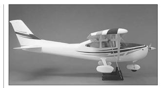
□ 2. With the wing attached to the fuselage, all parts of the model installed (ready to fly) and an empty fuel tank, place the model on a Great Planes C.G. Machine, or lift it at the balance point you marked.
