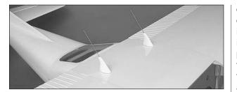
□ 3. The antenna bases fit into the wing bolt holes and are held securely in place with magnets.
