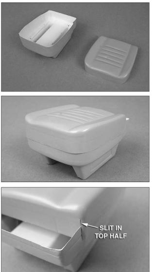
□ 2. Begin by cutting out the seat bottoms for the front seats. Canopy scissors work well for this. There are cut lines on the parts. However, we suggest cutting approximately 1/4" [6mm] beyond the cut lines and assembling the halves by overlapping the edges. (If you choose, you could cut along the cut lines and edge glue the two halves together. Because the pieces come pre-painted, a good fit would be difficult doing it this way). Small slits will need to be
