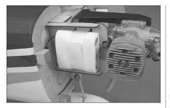
□ 2. Install the battery pack for the lighting system in the same manner on the other side of the motor mounting box.
