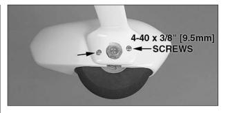
□ 4. Loosely thread a 6-32 x 1/4" [6mm] SHCS into each wheel collar along with threadlocking compound. Reinstall the wheel collars and wheels onto the axles and tighten the SHCS against the flat spots. Confirm that the wheels spin freely on the axles. Oil the axles as necessary. Install the wheel pants onto the main landing gear legs using 4-40 x 3/8" [9.5mm] machine screws and threadlocking compound.
