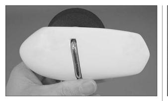
G. Insert the nose gear wire into the front wheel pant as shown. Slide a 5.5mm wheel collar onto the nose gear wire followed by the 2-3/4" [70mm] nose wheel, and another 5.5mm wheel collar. Center the wheel in the pant and mark the location of the wheel collars onto the nose gear axle. As you did with the main landing gear, file flat spots at the marks you made.
