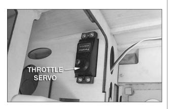
☐ 7. Install the throttle servo in the location shown. Because of the tight working space here, a Hobbico Pin Vise (HCAR0696) is very useful in this step. Use the hardware included with the servo.
