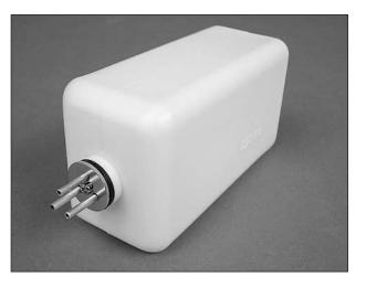
□ 2. Fit the stopper assembly into the tank with the vent line pointing toward the top of the tank, but not touching. The fuel tubing and clunks (fuel pickup) on the carb and fill lines should almost reach the back of the tank but not touch. The clunks must be able to move freely inside the tank when assembled.
