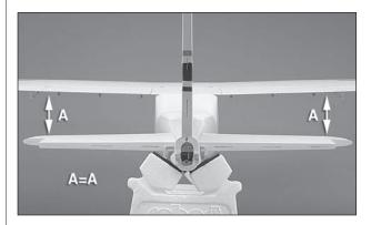
□ 1. Temporarily attach the wing to the **fuselage** using two 1/4-20 nylon wing bolts. The nylon wing dowels fit into receiving holes in the former just behind the location of the windshield. Test fit the **horizontal stabilizer** into the saddle in the fuselage. The beveled TE on the stab should slope forward from the top of the stab to the bottom. If not, the stab is installed
