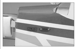
□ 6. Install your receiver switch and charge jack on the side of your fuselage. Be sure that the location you choose will not interfere with servos, pushrods, or the cockpit (look ahead in the manual to see the position of the cockpit kit components).
