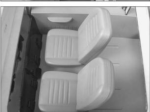
□ 11. Glue the seats to the cockpit floor. Remember, the seats should also be removable in case the floor needs to be taken out. Hot glue works well for this. Small dots of medium or thick CA could also be used.
