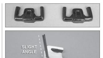
□ 9. Cut out the steering yokes and sand the bottom edges smooth. Fill the inside center of the yokes with epoxy and embed the included  $1/8" \times 1-1/2"$  [3 x 38mm] dowel rods into the epoxy. Set them at a slight angle as shown. Just as the epoxy begins to get hot and harden, hold the dowels in the desired position while the epoxy finishes hardening.
