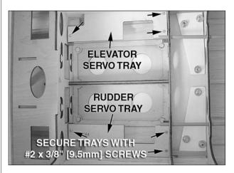
□ 1. Position the **elevator** and **rudder servo trays** onto the hardwood rails glued inside the fuselage as shown. Drill through the mounting holes in the trays into the hardwood rails using a 1/16" [1.6mm] drill bit. Thread a  $#2 \times 3/8$ " [9.5mm] self-tapping screw into each hole and back it out. Apply a drop of thin CA to each hole and let it harden. Install the trays into the fuselage using six  $#2 \times 3/8$ " [9.5mm] self-tapping screws.
