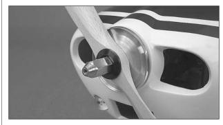
□ 2. Ream your prop as necessary. Install the spinner backplate, propeller, propeller washer and spinner nut onto the engine crankshaft. If you installed a four-stroke engine, use the four-stroke spinner nut.
