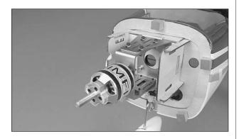
□ 2. Attach the mount to the firewall on its side using four 8-32 x 1" [25mm] SHCS, four #8 flat washers, four #8 lock washers and threadlocking compound.
