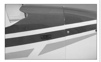
□ 5. Install the included switch for the landing lights (be sure that the charge lead remains accessible). Connect the included 3-way parallel connector to the two lights in the cowl and the wire leading from the beacon light in the tail. Join the lights to the switch and connect the light battery to the switch. Confirm the operation of the lights by flipping the switch on and off.
