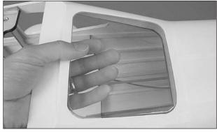
□ 2. Use canopy scissors to trim the rear window to size. Leave a gluing flange around the window approximately 1/8" [3.2mm] wide. Glue the rear window in place. If canopy glue is used, you will need to tape the window in place and temporarily glue a stick on the inside of the window to hold it against the window opening while the glue dries overnight.
