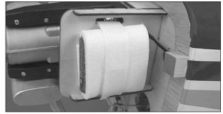
□ 1. Make a hook and loop strap for your receiver pack from the included hook and loop material by overlapping mating ends by approximately 1" [25mm]. The total length of the strap will depend on the size of your battery. Wrap the pack in foam rubber (not included) and use the strap to secure it to the side of the motor mounting box as shown.
