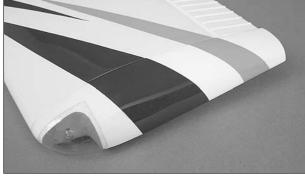
□ 1. Sand the inside face of the **wing tips** with 220-grit sandpaper. Clean the surfaces with a cloth dampened with denatured alcohol. As you did with the ailerons, use the string to pull the wingtip light wires through the wing panels. Use epoxy to glue the wing tips to the wing, being sure that the curved tips point to the **underside** of the wing. Align the tops and bottoms of the wing tips flush with the wing and the LE of the tips in position while the epoxy cures.
