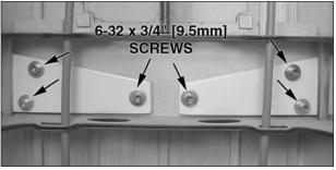
□ 5. Insert the landing gear legs into the slots in the fuselage. Attach the gear to the fuselage using six  $6-32 \times 3/4$ " [19mm] SHCS, six #6 flat washers, six #6 lock washers, and threadlocking compound.
