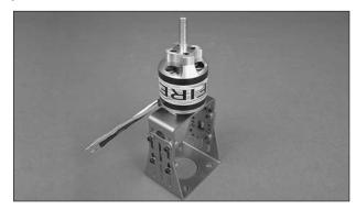
$\Box$  1. Attach the motor to the brushless motor mount using four 3 x 8mm machine screws, four 3mm flat washers, and threadlocking compound. You may need to remove the brass collar to fit the motor to the mount. Be sure and replace the collar after the motor is installed. If you haven't done so already, install the prop adapter to the front of the motor using the hardware included with the motor and threadlocking compound.
