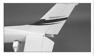
□ 6. As you did with the elevators, install the rudder to the fin with CA hinges.
