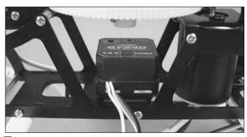
☐ 3. Install the gyro directly under the main shaft. Connect your rudder servo to the gyro's output port.
