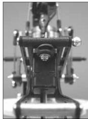
7. Install the aileron servo using the hardware that came with your servo. If using the recommended Futaba servo, you will need to install the metal eyelets upside-down and install the servo under the tray, with the screws running up into the tray.
