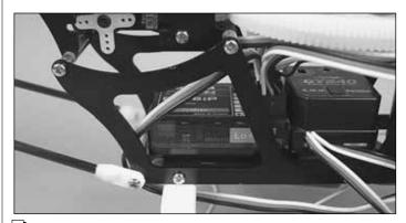
4. Install the receiver in the position shown. Connect your servos and gyro to the appropriate channels.
