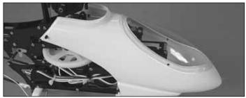
☐ 12. Install the canopy onto the helicopter.
