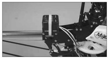
Alternately, the gyro can be installed on top of the rear end of the main frames. Use a piece of foam tape to isolate the gyro against vibration, and secure it with a tie wrap. An optional mount (HMXE7921) is available.
