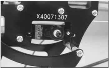
4. Install the rudder servo as shown, using the hardware that came with your servo and two plastic servo nuts. The servo mounting lugs should be on the outside of the frame.
