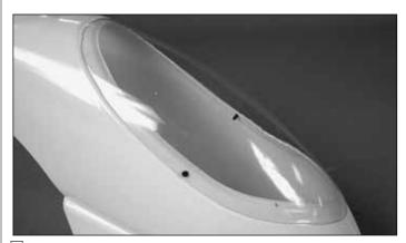
11. Secure the shield to the canopy with the two small screws packaged with the shield.
