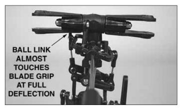
To set rates on the elevator and aileron, check to see that the control rates are set to maximum for high rates. This can be verified by checking that the ball link attached to the seesaw is close to touching the main rotor grips at full input. Check the elevator rate with the flybar perpendicular to the tailboom, and check the aileron rate with the flybar parallel to the tailboom. These maximum deflections work well for high rates, and we recommend 60% of these values for low rates.
