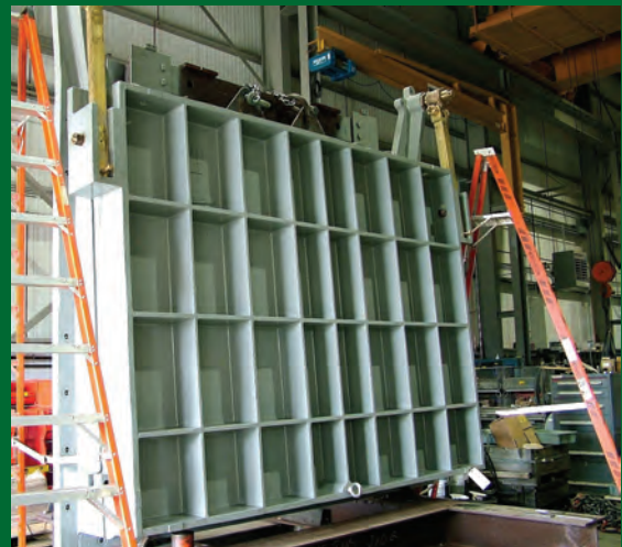
Ally Creek-East River, Queens, NY – Four 120" x 90" (3050mm x 2290mm) Flap Gates with neoprene resilient seats
