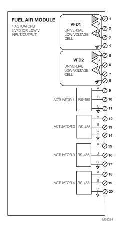
Fig. 3. Wiring diagram for Fuel Air Ratio Module.
