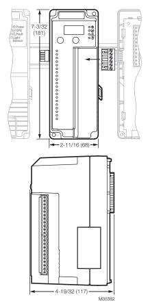
Fig. 1. Dimensions in in. (mm).
