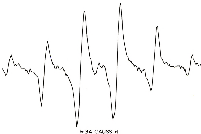
Fig. 2. Electron spin resonance spectrum of irradiated solution-crystallized polyethylene. Magnetic field parallel to chains.
