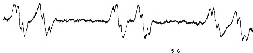
Figure 1. EPR spectrum of the spin adduct in \gamma irradiated 0.1 M phenyl tert -butyl nitron in acetonitrile ( \text{CH}_3\text{CN} ) at room temperature at 0.2 Mrad dose in benzene solvent. The spectrum is assigned to the \cdot\text{CH}_2\text{CN} adduct.
