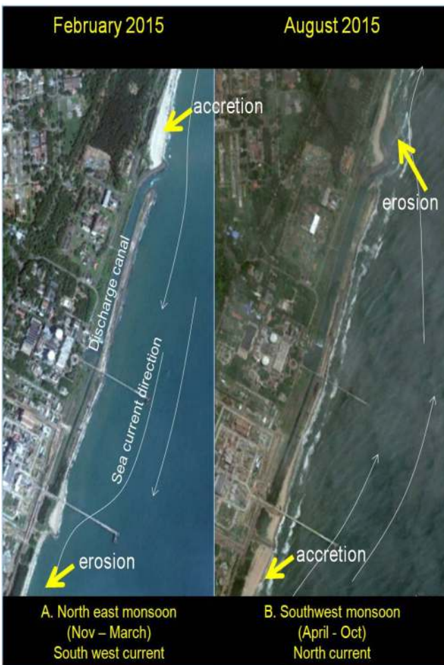
Fig. 8.13: Sediment accretion-erosion pattern along combined PFBR-MAPS discharge canal with respect to season
