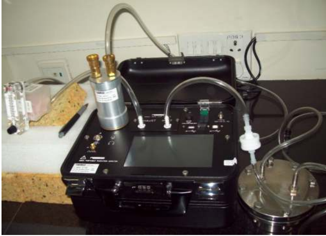
Fig.8.14: Determination of radon concentration using Radon Monitor
