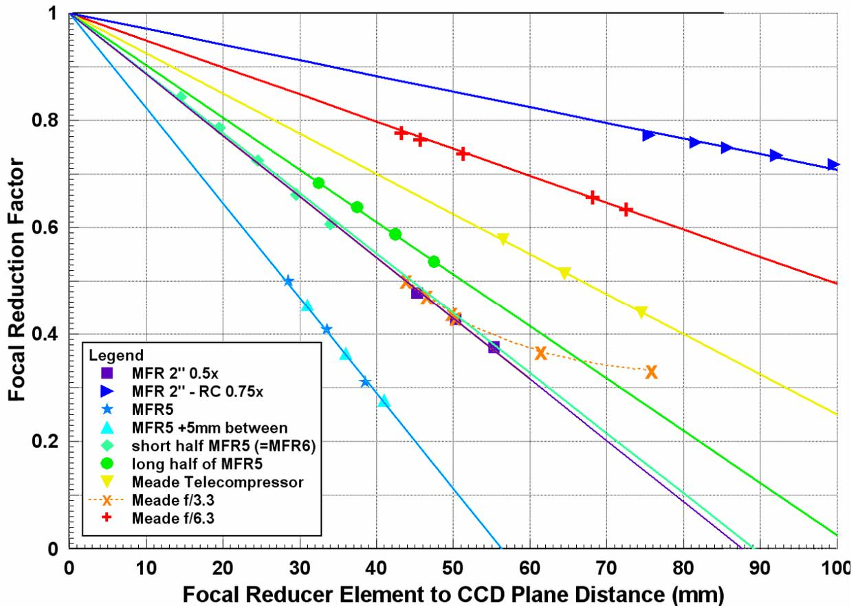
Figure 2 Measured Focal Reduction Factor vs. FR-to-CCD Distance
