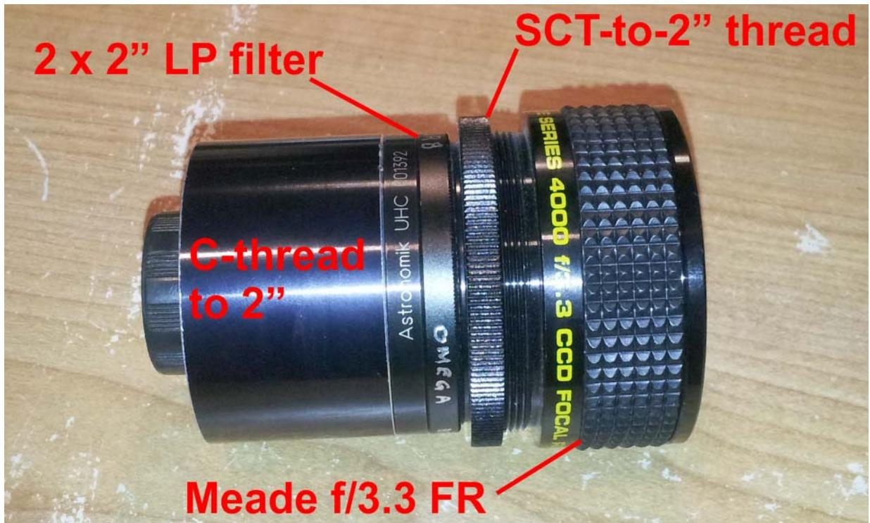
Figure 17 Final Tested Meade f/3.3 FR Configuration
