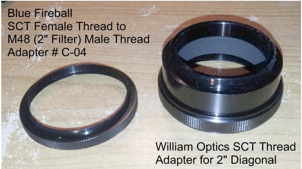
Figure 13 SCT-to-2" Adapters Used In Tests
