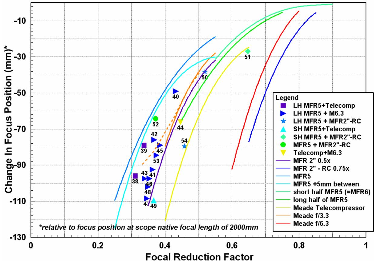
Figure 15 Compound FR Measured Focus Position Change vs. Focal Reduction Factor
