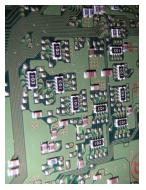
Another PCB in a DoD Platform; 20-pin ARIC with Resistors and Capacitors
