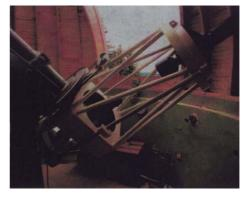
Fig. 3. The 60-cm photometric telescope.
