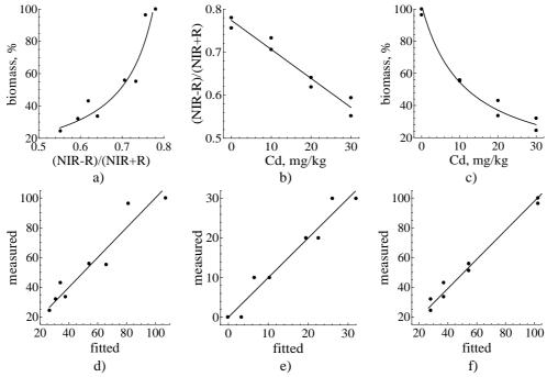
Fig.2 Relationships between peas plots spectral index (NIR-R)/(NIR+R), biomass (relative to the control treatment) and Cd contamination (a,b,c); correspondence between the actual and fitted (model) values of the bioparameter (d,f) and the stress factor (e) In Fig.3 the spectral index (NIR-R)/(NIR+R) temporal profiles of barley
