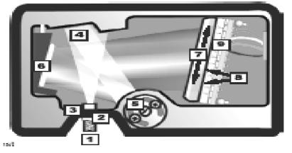
*Fig5. Diagram of the optical unit* 1. SMA connector; 2. Fixed slit; 3. Absorbance filter; 4. Collimating mirror; 5. Grating; 6. Focusing mirror; 7. Detector collection lens 8. OVLF filter; 9. UV detector.
