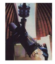
Fig.4. The 50/70 cm Schmidt telescope.
