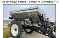
BBI Magna Spreader. High clearance spreader for In season or Out of season applications 12' Bed capable 120' spread pattern
